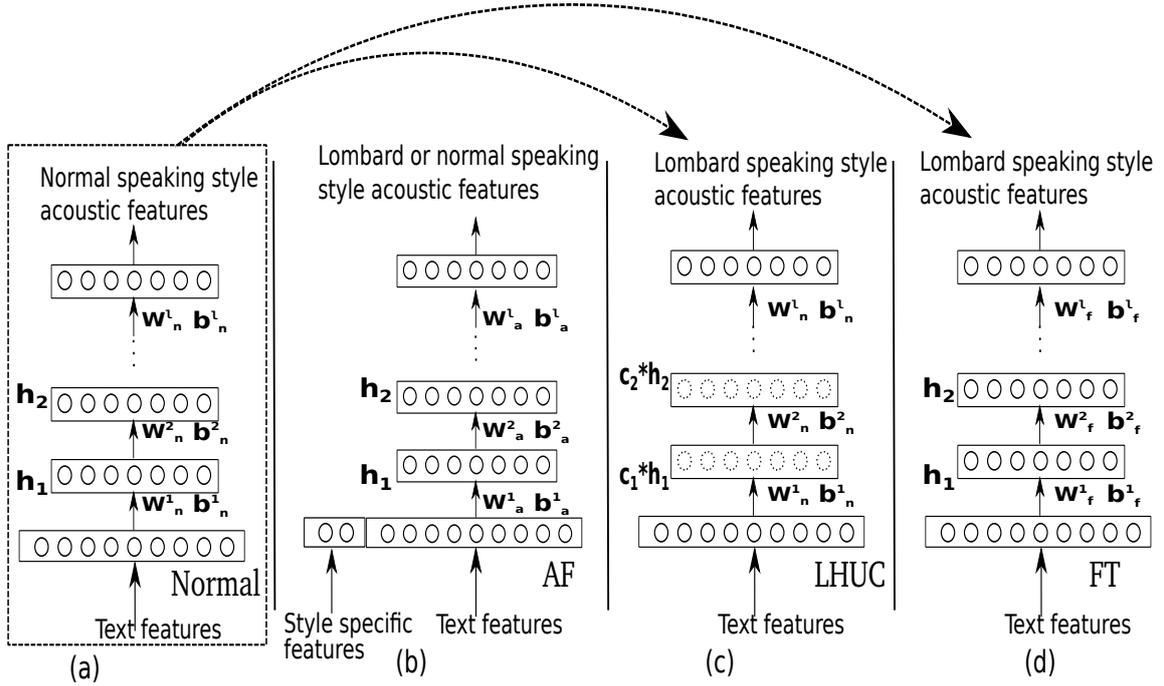
Fig. 2. Illustration of the synthesis systems compared. (a) Normal speaking style TTS system. Adapted systems based on (b) auxiliary features (AF), (c) learning hidden contribution (LHUC), and (d) fine-tuning (FT). Adapted systems LHUC and AF use the normal speaking style TTS system as an initial system.
