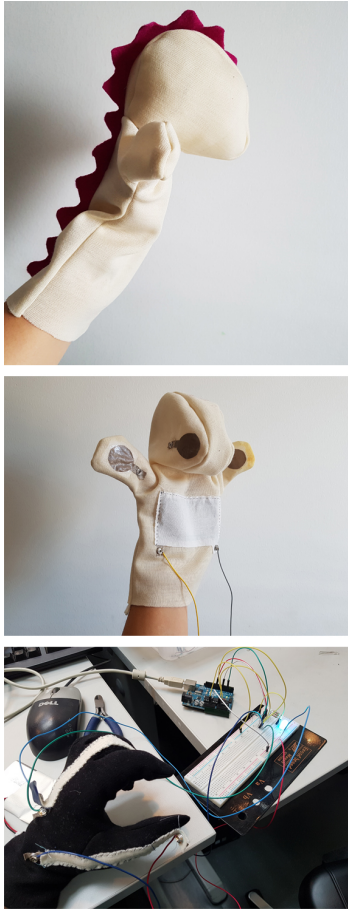
Figure 2: Prototyping eTextiles. From the top down: a non-functional prototype of the hand puppet, a functional prototype of the outer layer, and a functional prototype of the inner glove.
