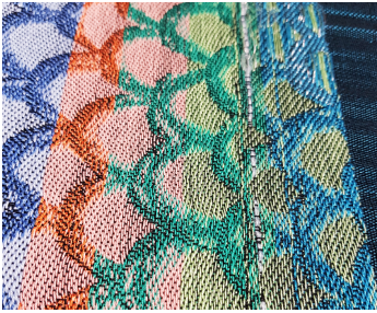
Figure 4: A colour and bind test
