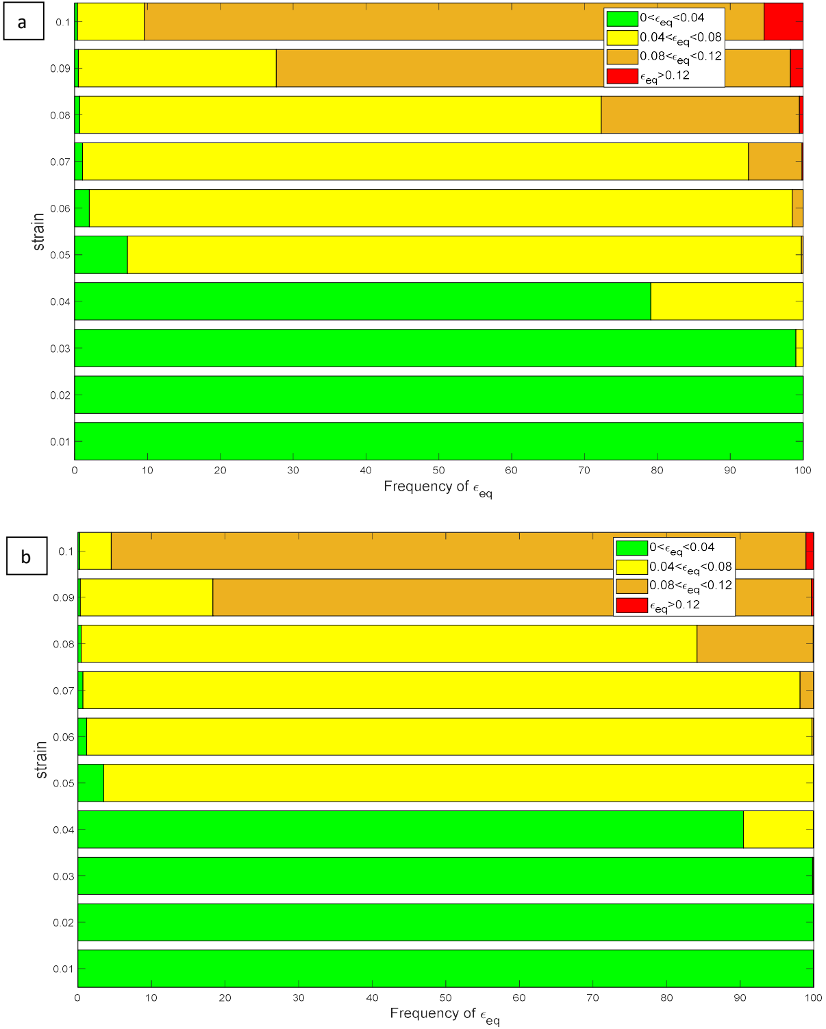
Fig. 8. The evolution of equivalent plastic strain at different strain state for composites extruded at (a) 600 psi and (b) 750 psi.
