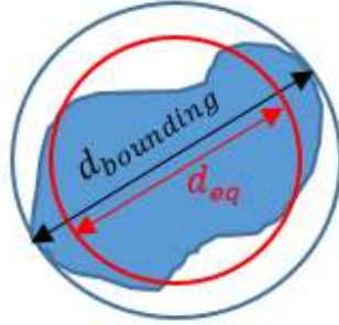
Fig. 3. Bounding sphere diameter ( d_{bounding} ) and equivalent spherical diameter of cluster ( d_{eq} ).
