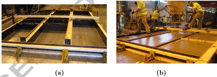
**Fig. 1.** Casting of full-size floor-slabs in a factory. (a) Representation of the formwork with surface treatment. (b) Representation of the way of casting.
