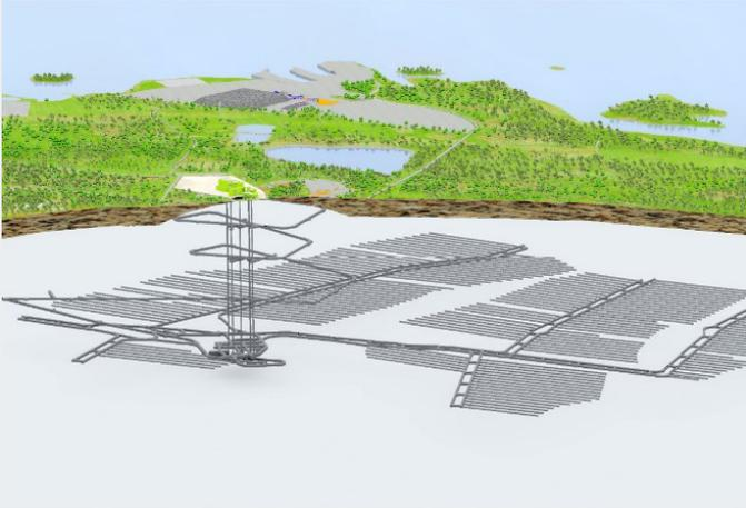
Repository for highly radioactive waste (Olkiluoto Posiva). Magnification of one horizontal tunnel with deposition holes for canisters is shown at left.
