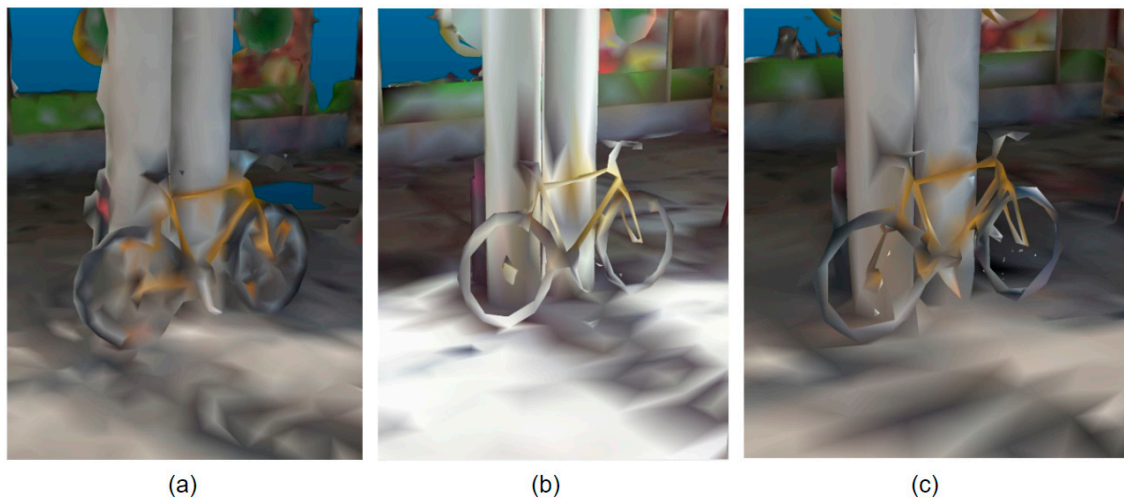
Figure 5. Visual comparison of details in (a) photogrammetry; (b) TLS; and (c) hybrid approaches. The photogrammetry model suffers from blurred details, whereas the texture data of the TLS model suffers from clear overexposure. For visualization purpose, the models are visualized here as colored vertices without the textures.
