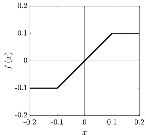
Fig. 9. Hard-clipping waveshaper transfer function with the threshold parameter set to 0.1.
