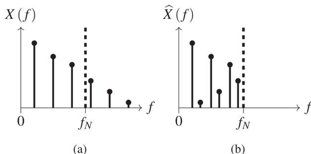
Fig. 1. Aliasing understood as mirroring alongside the Nyquist limit ( $f_N$ ): (a) the generation of harmonics in the spectrum of a signal that exceed the Nyquist limit (dashed line) leads to (b) their reflection around the Nyquist limit, when sampled.
