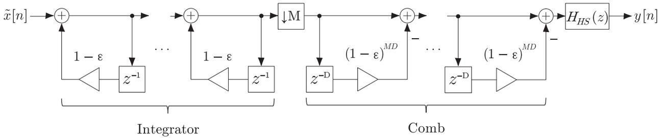
Fig. 5. Architecture of the decimation block when considering the CIC filter, which consists of a leaky CIC decimation filter cascaded with a first-order high shelving filter:  $\tilde{x}[n]$  is the signal that enters the decimation filter (after having been interpolated and waveshaped) and  $y[n]$  is the resulting output. Figure based on [22, 26, 30, 31].
