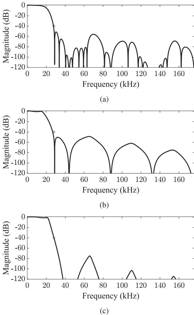
Fig. 7. Cascaded magnitude responses of the linear interpolator with the (a) IFIR, (b) elliptic, and (c) CIC decimation filters for the oversampling factor  $M = 8$ . The corner of the stopband at 28.1 kHz and at  $-40$  dB is indicated with a cross (+).
