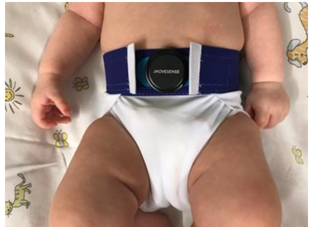
Figure 4: B) The first prototype for detecting sleep cycles. Photo by Natalia Acosta.
