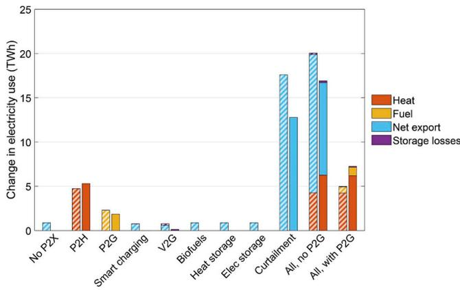
**Fig. 6.** Change in electricity use compared to the reference case (Finland 2030). The columns on the left (striped) refer to constant CHP, and on the right (solid) to variable CHP.
