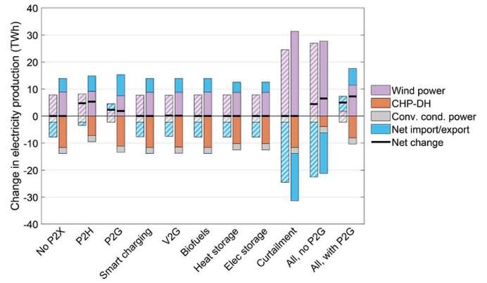
**Fig. 4.** Change in electricity production compared to the reference case (Finland 2030). The columns on the left (striped) refer to constant CHP, and on the right (solid) to variable CHP.
