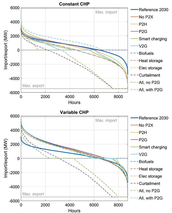
**Fig. 7.** Duration curve of power import (positive) and export (negative) with the different flexibility measures, with (a) constant CHP and (b) variable CHP.
