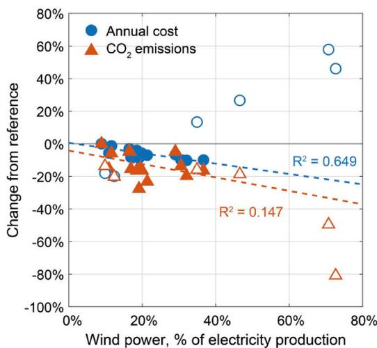
**Fig. 9.** Relative annual cost and CO<sub>2</sub> emissions against the share of wind power in all cases. The linear trend lines consider only the original scenarios (filled points), whereas the unfilled points represent the special scenarios with variable nuclear power (original nuclear cost) and wind maximization. Annual cost presents a clear downward trend with increasing wind power in the original scenarios.
