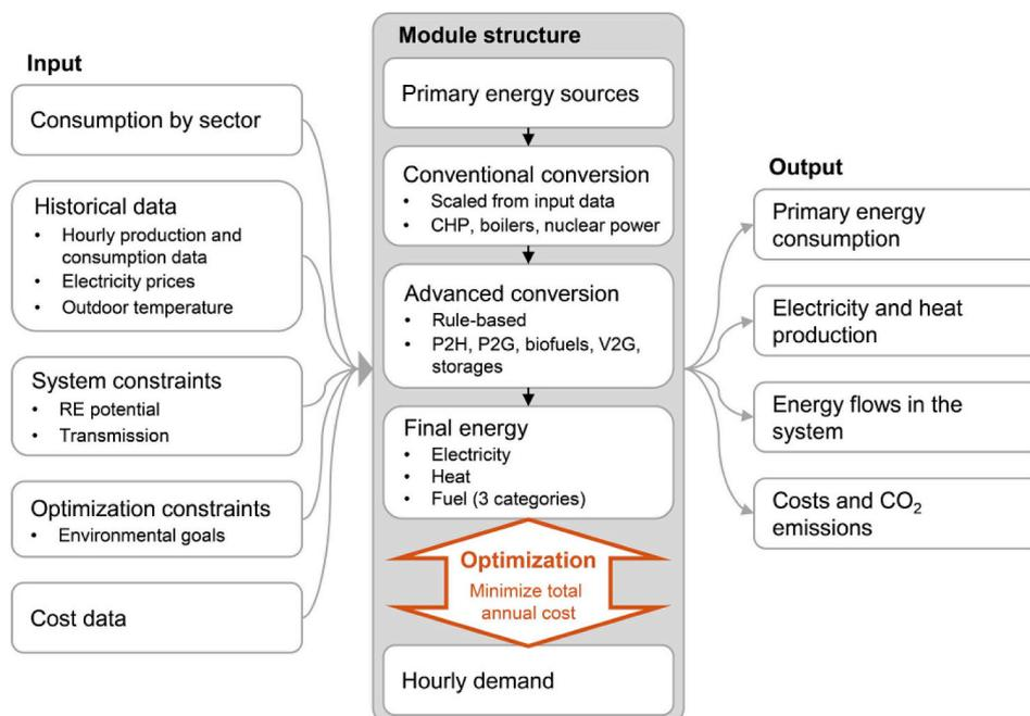
Fig. 1. Schematic of the modelling approach.
