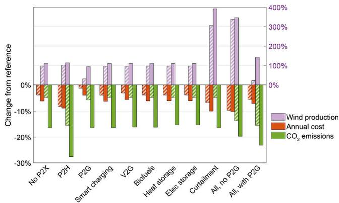
Fig. 8. Effect of the different flexibility measures as change from the reference case (Finland 2030). Power-to-heat (P2H) and curtailment are the most cost-effective options, though the cost differences are quite small, max. 10% from the reference case. The columns on the left (striped) refer to constant CHP, and on the right (solid) to variable CHP.
