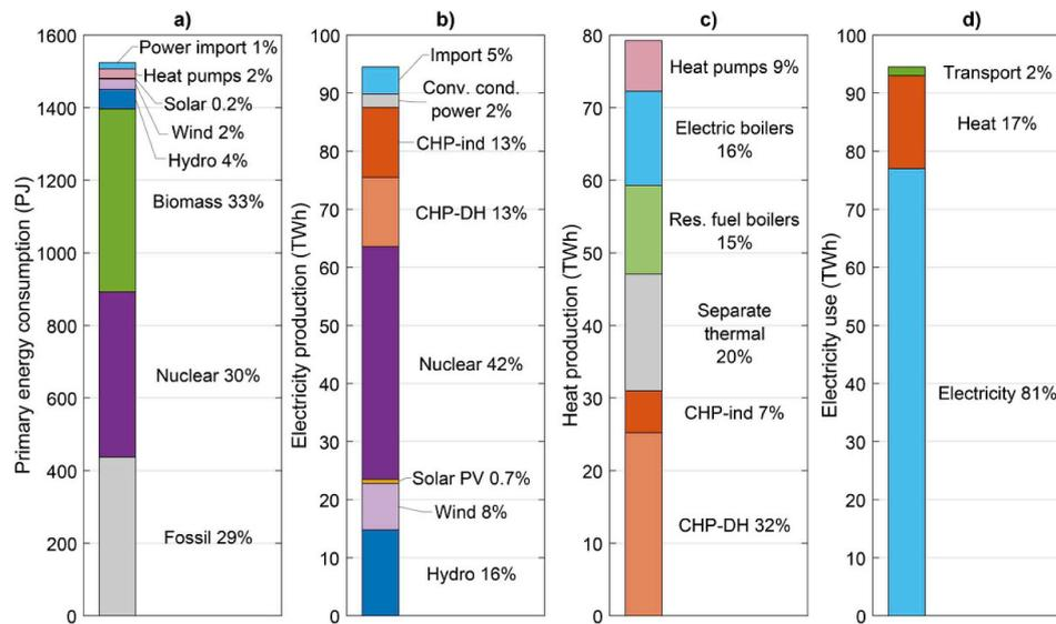
Fig. 2. Reference scenario (Finland 2030) based on the National Energy and Climate Strategy 2030 [31]. (a) Primary energy consumption (b) Electricity production (c) Heat production (d) Electricity use.
