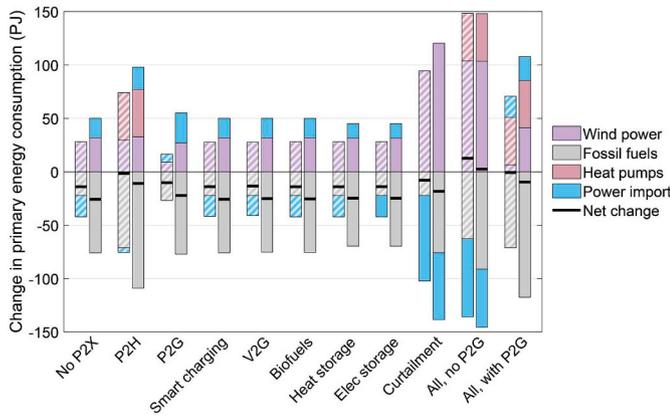
**Fig. 3.** Change in primary energy compared to the reference case (Finland 2030). The columns on the left (striped) refer to constant CHP, and on the right (solid) to variable CHP.
