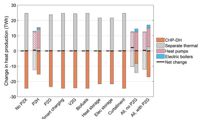
**Fig. 5.** Change in heat production compared to the reference case (Finland 2030). The columns on the left (striped) refer to constant CHP, and on the right (solid) to variable CHP.
