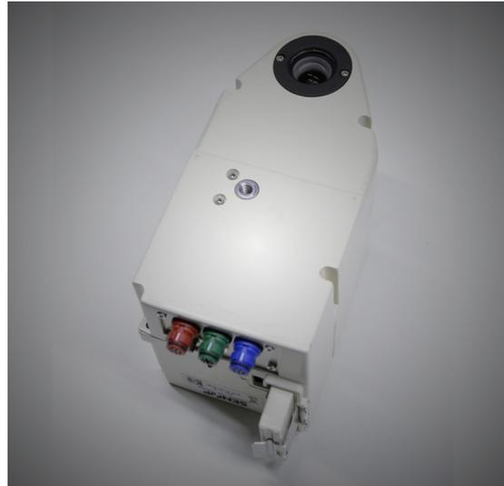
**Figure 1.** Photograph of the hyperspectral camera used in the study, with strong artificial vignetting effect added to the image.
