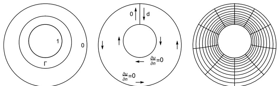
(a) Ring domain with boundary conditions.  $\Gamma$  is one of the contours, i.e., equipotential curves of the solution  $u$ .
