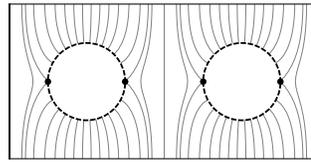
(b)  $Q$ -type. Contour plot of  $u$ . Dirichlet on left ( $u = 0$ ) and right ( $u = 1$ ). Neumann zero-condition on other boundaries. Locations of maxima and minima on the interior boundaries are indicated.
