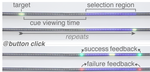
Figure 5: The task in Study 1, to select a moving target within the selection region by clicking a button, as the target moved from left to right.
