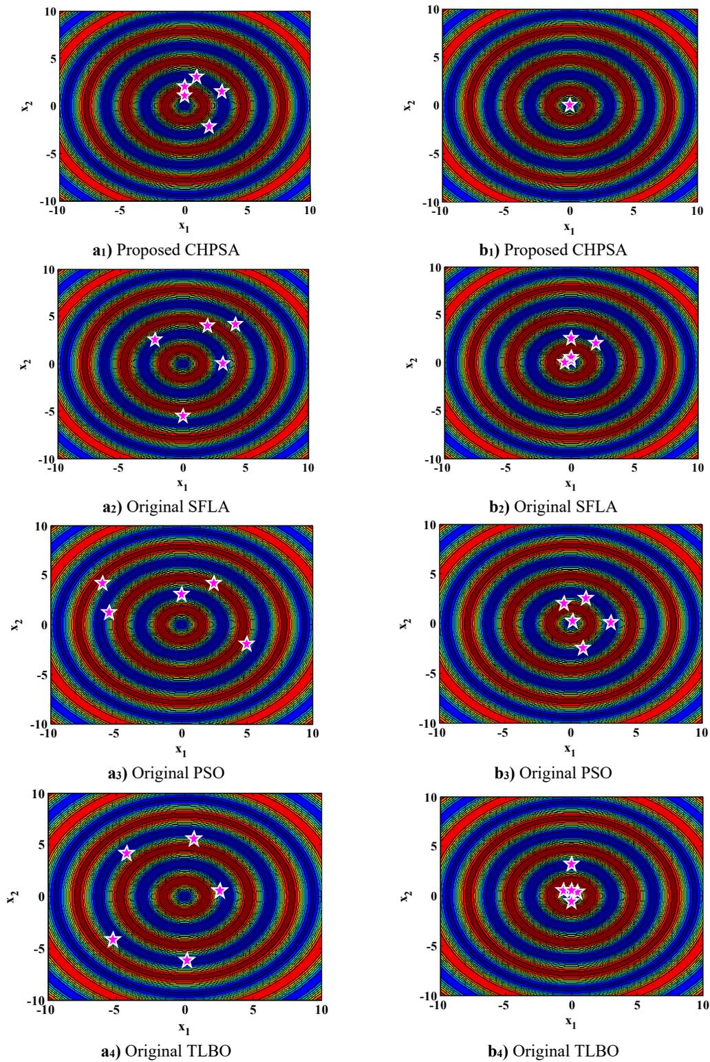
Fig. 7. Obtained results of different algorithms for minimizing the Schaffer's function; **a)** After the first iteration, and **b)** After the final iteration
