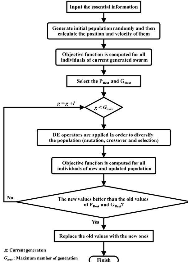
Fig. A5. Hybridization process of MPSO and DE algorithms in this paper
