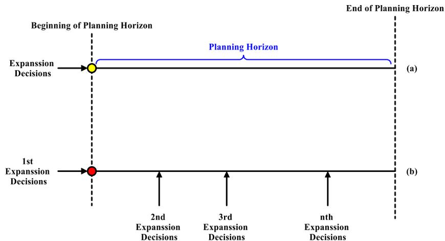
Fig. A1. Comparison of common models in solving the TEP problem, (a) Static or single-stage TEP, and (b) Dynamic or multi-stage TEP
