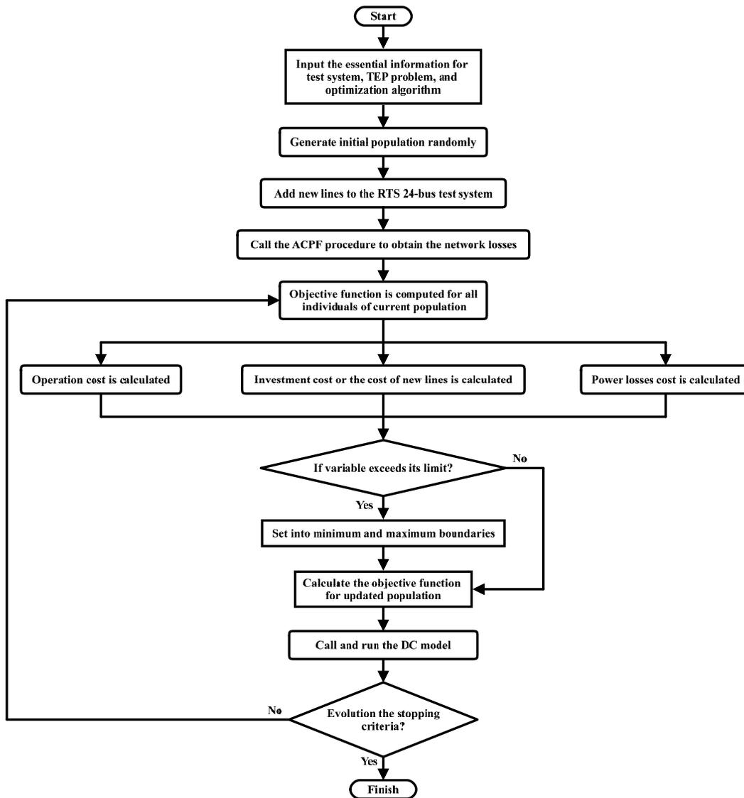
Fig. 4. The flowchart of solving the proposed TEP problem in this paper
