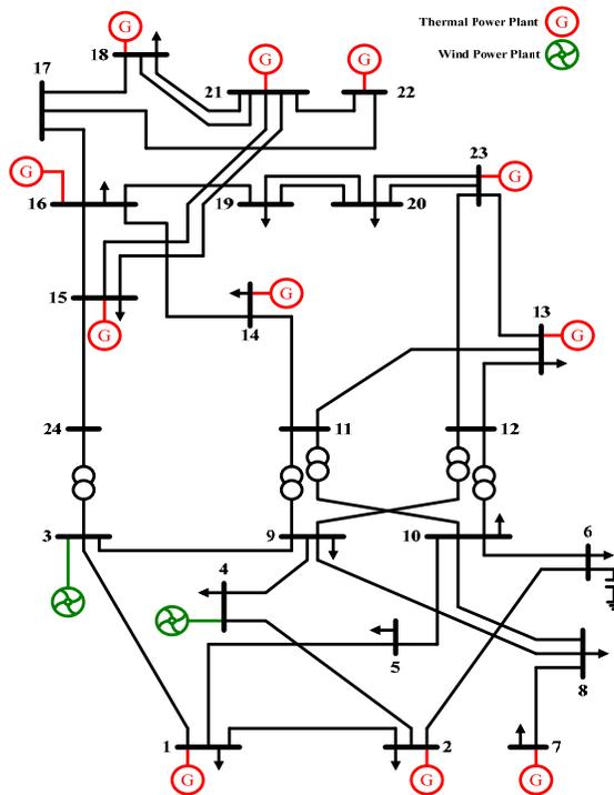
Fig. 8. Single-line diagram of IEEE RTS 24-bus test system including two wind power units
