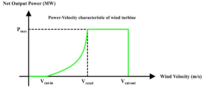
Fig. 2. The curve of wind turbine power output versus wind velocity
