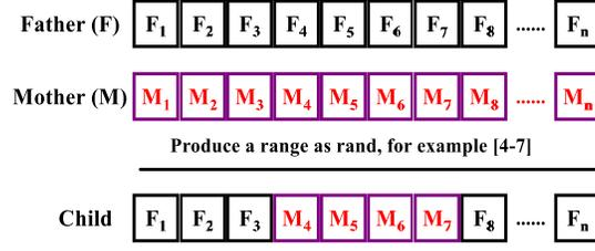
Fig. A2. Operation of crossover in order to produce the new child in offspring process
