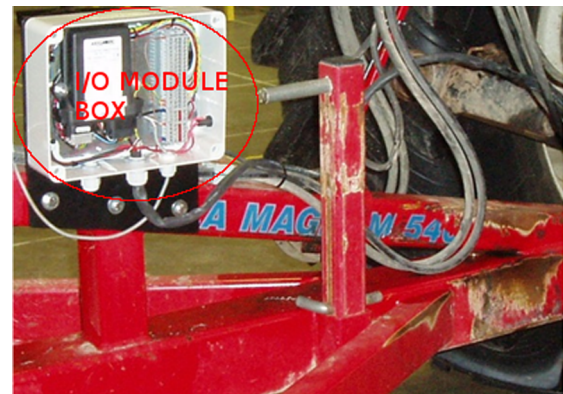
Fig. 6. In figure I/O module fitted to Potila Magnum 540 harrow.
