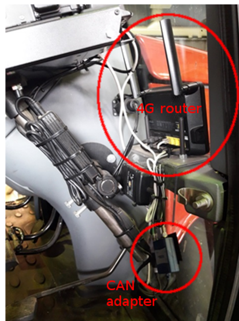
Fig. 10. Wireless 4G router is used to cloud connection and national instruments CAN-adapter for ISOBUS connection.
