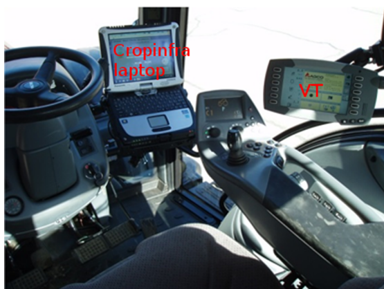
Fig. 9. Rugged computer for data capturing is mounted in the tractor.
