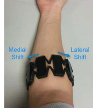
Figure 2. Myo Armband placement on the right forearm of a subject. The transversal shifts of 1cm along the indicated directions have been induced in order to simulate prosthetic donning and doffing.
