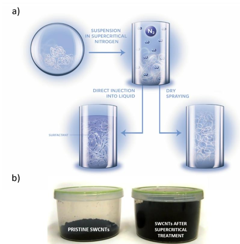
**Figure 1.** a) Schematic diagram of two methods: direct injection into liquid, leading to the formation of the SWCNT dispersion, and dry spraying method, resulting in the loose
