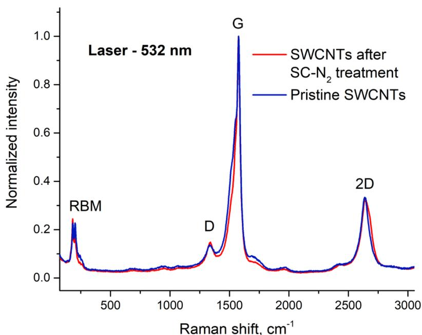
**Figure 2.** Raman spectra of pristine SWCNTs and tubes after the supercritical nitrogen treatment (a dry spraying method).
