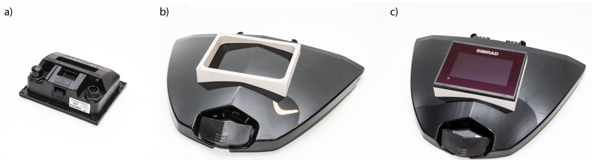
Figure 6: The underside of the chart-plotter unit that is to be mounted (a). The adapter component had to match the flat underside of the plotter flange to the curved surface of the fairing (b). The completed assembly (c).
