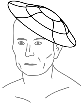
Figure 1: An example of an overall coil shape with one surface with a flat central part and a curved exterior part.
