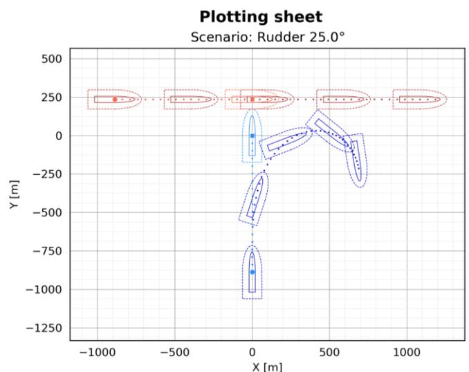
Figure 2 - Example plotting sheet with ships' hulls and safety margin projection.
