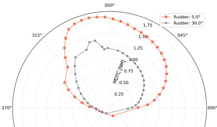
**Figure 4 – CADCA envelope for two extreme rudder angles presented for the bearings to the target.**
