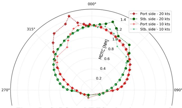
Figure 7 – CADCA as MDTC vs bearing to target for both turning sides. Rudder angle 25°, speed 10 and 20 kts.
