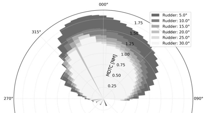
**Figure 3 – CADCA for 6 various rudder angles presented for the bearings to the target.**
