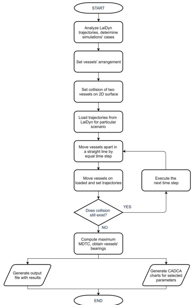
Figure 1 - Flowchart of CADCA simulator.
