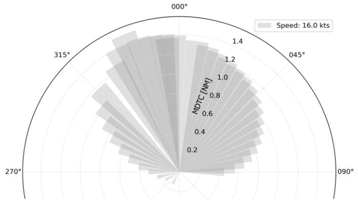
**Figure 6 - MDTC vs bearing to the target for initial speeds 16 kts of both vessels.**
