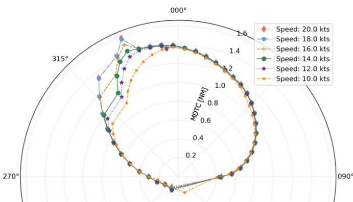
**Figure 5 – CADCA presented as MDTC vs bearing to the target for various initial speeds of both vessels.**
