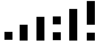
Fig. 4. Close-up on a bitmap generated after static mode tests and showing the shape of single word errors or small cluster of errors.
