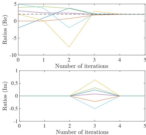
Fig. 2. Average consensus is reached for the ratio  $y_j[k]/x_j[k]$  of each node  $v_j$  for a digraph of size 6 in 5 steps. The *top figure* shows the evolution of the real part of the state of each node  $v_j$  and the *bottom figure* shows the evolution of the imaginary part of the state of each node  $v_j$ .
