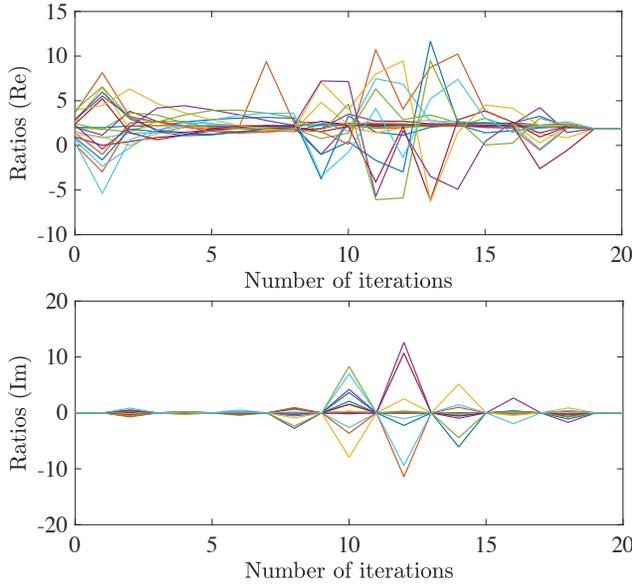
Fig. 5. Average consensus is reached for the ratio  $y_j[k]/x_j[k]$  of each node  $v_j$  for a digraph of size 20 in 19 steps.
