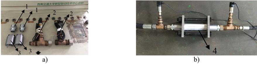
Fig. 4. Experimental devices of SEC and DTETC: 1 – union joints, 2 – pressure sensors, 3 – inserted tubes, 4 – expansion chamber cavity
