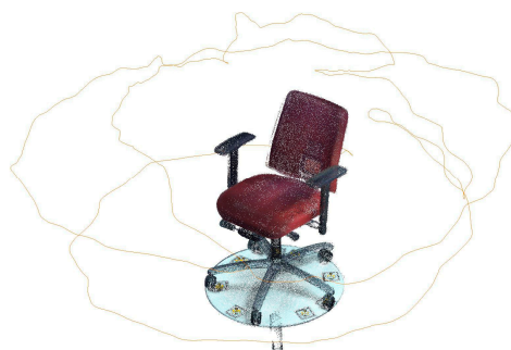
Figure 5. An object point cloud reconstructed with a hand-held scanner shown with the measurement trajectory and automatically detected markers mounted adjacent to the object on the table surface.
