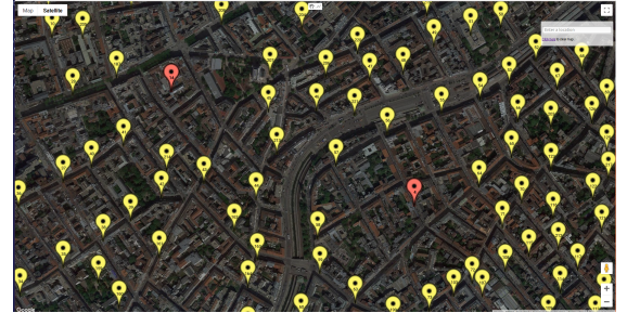
Fig. 1: Assumed network deployment in Vienna city. Macro BSs are denoted by red and small BSs by yellow markers.
