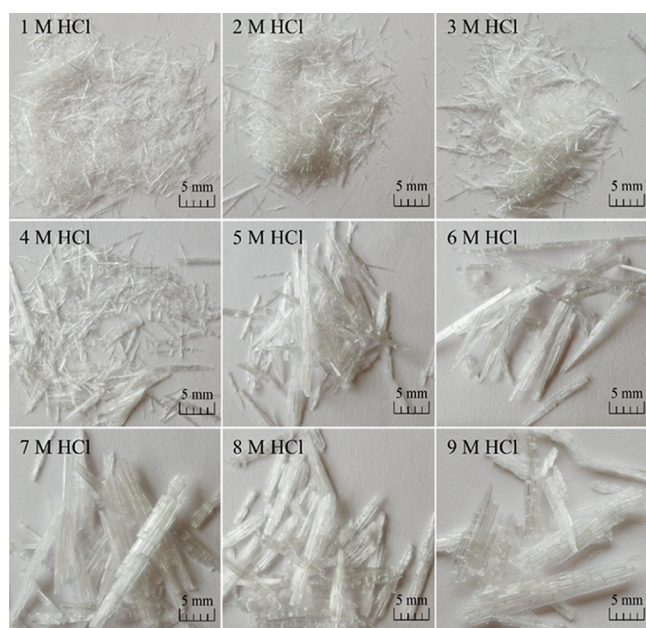
Figure 5. Morphology of oxalic acid products at different HCl concentrations ( t = 2 h, T = 5 °C).
