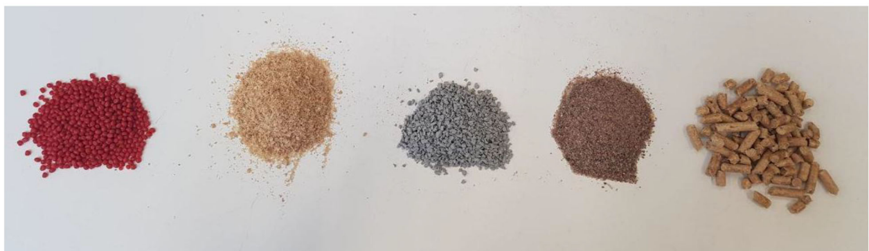
Fig. 3. Five different types of granular materials starting from the left: plastic granules, ground wooden pellets, rubber granules, fine sand; and wooden pellets.
