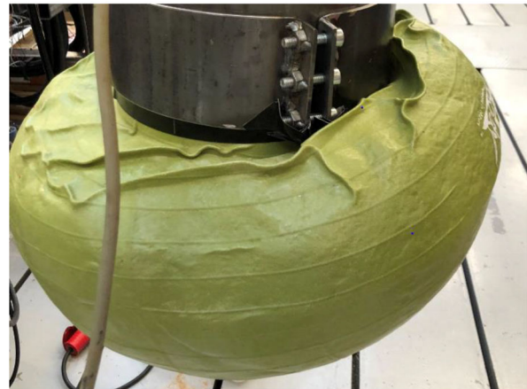
Fig. 6. Large wrinkles forming on the gripper's surface, when the gripper with ground wooden pellets as granular material was evacuated of air.
