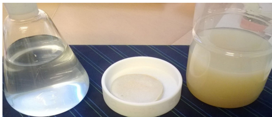
Fig. 5 The suspension of TLNP50 after reaction with allylated cellulose fibres (left), the filtrated suspension on a filter paper sheet (middle), and the clear filtrate of suspension (right)
