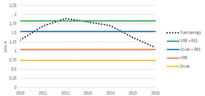
Figure 6. Potential fuel saving and costs of employing 4 MW flow battery, along with 4.5 MW wind park and 1 MW solar farm, on Graciosa.
