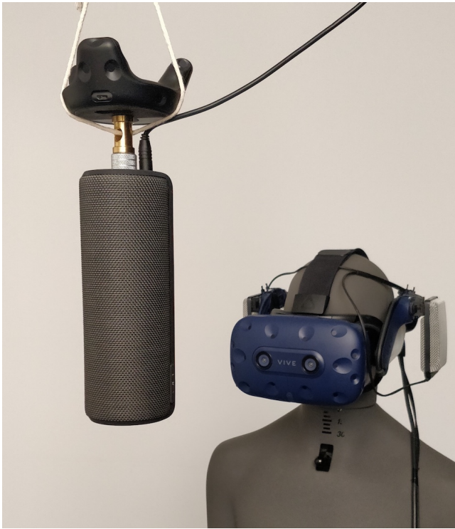
Figure 3: Cortex Mk I dummy-head during calibration and the ceiling-suspended loudspeaker with a tracker mounted on top. The dummy-head is wearing an HTC Vive Pro HMD and the AKG K1000 open-design headphones.
