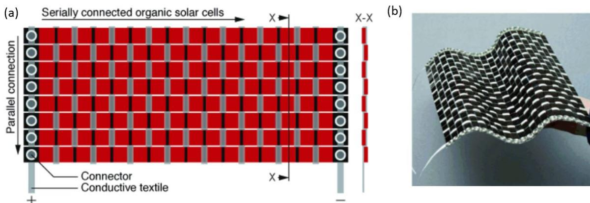
Figure 7. a) Structure of the tape-weaved solar cell textile reported by Krebs and Hösel (2015), and b) a photograph of one of their large area (25 x 25 cm<sup>2</sup>) solar cell textile examples. The solar tapes weaved in the structure consisted of 16 serially connected single junction organic solar cells and had an active area of 368 cm<sup>2</sup> and efficiency of ca. 1%. Reproduced with permission from John Wiley and Sons (copyright).
