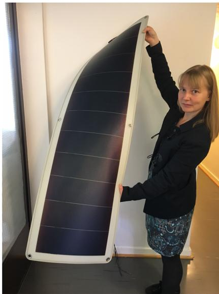
Figure 1. A flexible triple-junction a-Si PV module ( $32W_p$ ) from the 1990s.
