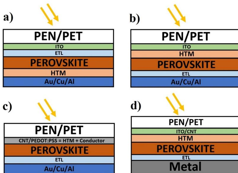
Figure 4. Popular configurations of perovskite solar cells on flexible substrates.
