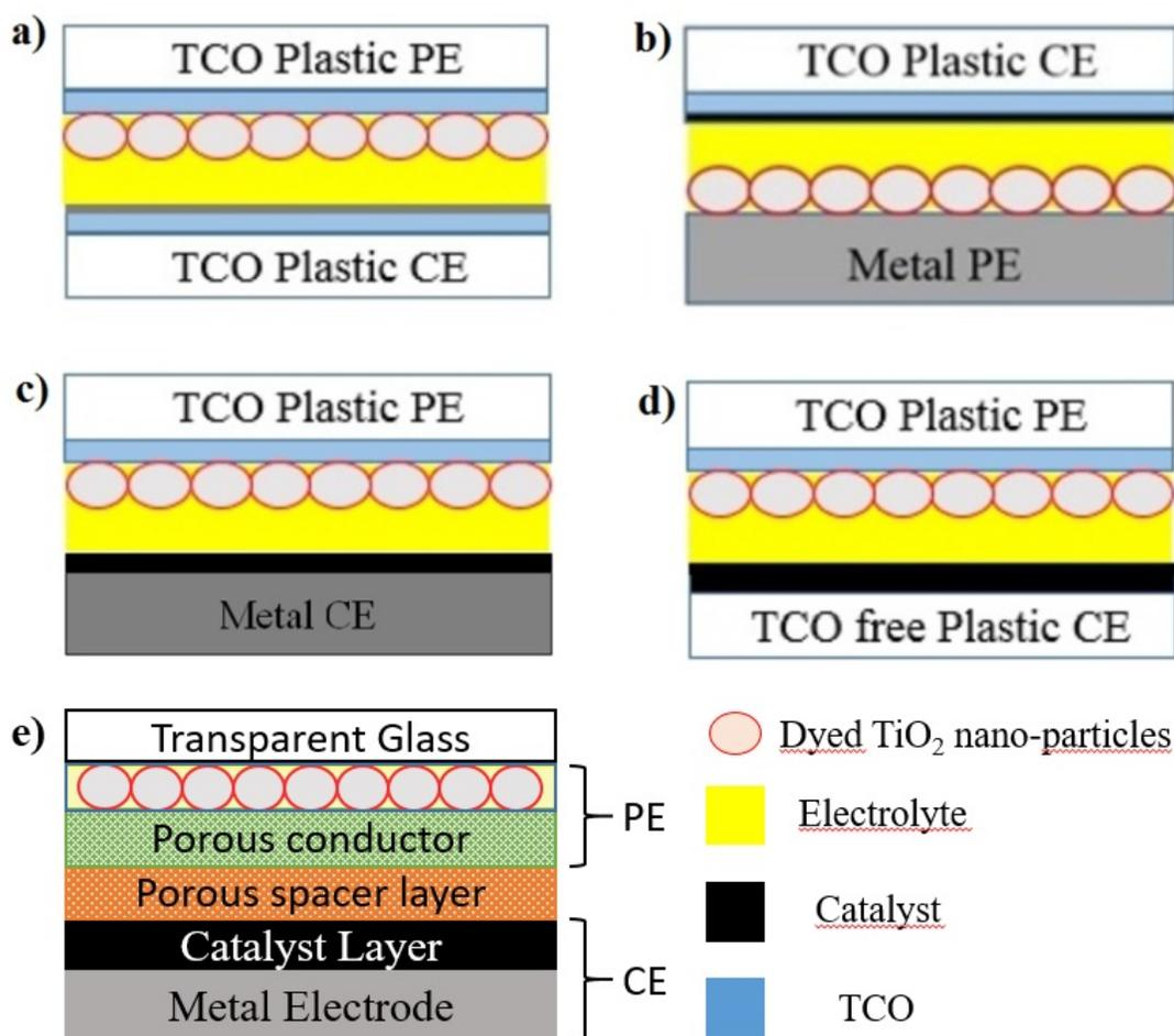
Figure 3. Different configurations of flexible DSCs. a) Traditional front illuminated DSC, b) Metal PE based reverse illuminated DSC, c) Front illuminated DSC with Plastic PE and Metal CE, d) Front illuminated DSC with Plastic PE and TCO free plastic CE, e) Flexible back contact DSC on metal substrate (PE =photo electrode, CE= counter electrode, TCO = Transparent conducting oxide such as tin-doped indium oxide or ITO Layer).
