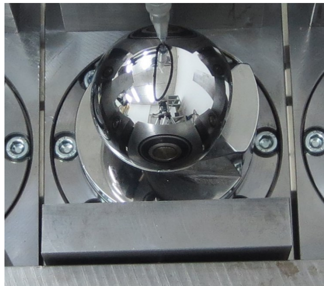
Fig. 4. Verification of force track in HUT-4 hip joint simulator using stationary pen on 54 mm diameter femoral head with three-axis motion according to ISO 14242-1. Simulator position as in Fig. 1.
