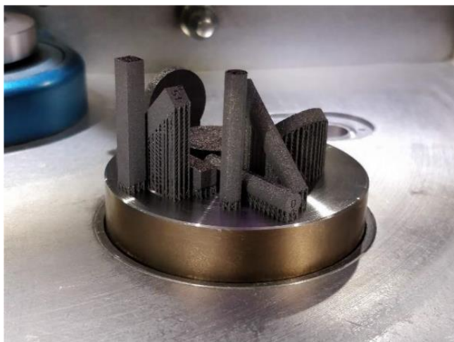
Fig. 3. First set of test samples: 3% Si to Fe printed in argon environment.
