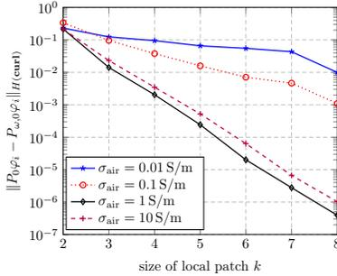
Fig. 3. The error  $\|P_0 \varphi_i - P_{\omega,0} \varphi_i\|_{H(\text{curl})}$  for  $\mu_c = 50$ ,  $\mu_{air} = 1$ ,  $\sigma_c = 100 \text{ S/m}$  and varying  $\sigma_{air}$  as a function of the neighborhood size.
