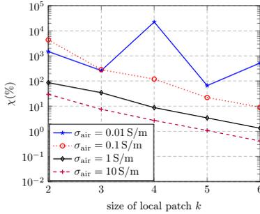
Fig. 4. The relative error  $\chi$  as a function of the neighborhood size. The same material parameters as in Fig. 3.
