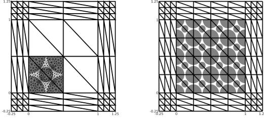
Fig. 2. On left: computational domain with  $2 \times 2$  cells. Coarse mesh  $\mathcal{T}_h$  of the whole domain is drawn together with the fine mesh for the cell  $[0, 0.5]^2$ . On Right: computational domain with  $4 \times 4$  SMC conductor. Dark gray denotes conductor with material parameters  $\mu_c, \sigma_c$ . Rest of the domain is air with material parameters  $\mu_{air}, \sigma_{air}$ .
