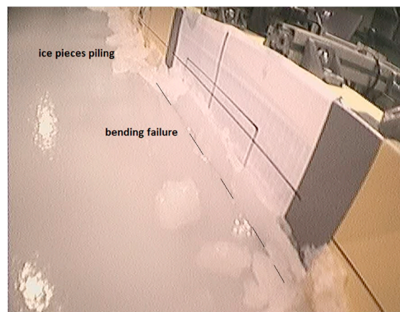
Fig. 4. A typical bending failure when a ship is moving in a compressive ice channel. The black dashed line illustrates the bending crack location (Source: Li et al. [28]).
