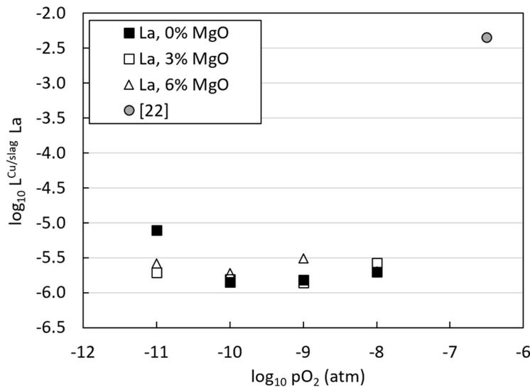
**Figure 6.** The distribution coefficient of lanthanum between copper alloy and molten slag. A result for neodymium (which behaves very similarly as lanthanum) from an earlier study [22] has been plotted for comparison.
