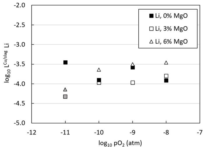
**Figure 5.** The distribution coefficient of lithium between copper alloy and molten slag. The values for MgO-containing slags in  $p(O_2) = 10^{-11}$  atm (grey triangle and square) have been calculated based on the detection limits in the copper alloy, as the concentrations were below detection limits of LA-ICP-MS in all analysis points.
