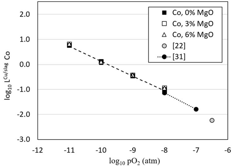
**Figure 8.** The distribution coefficient of cobalt between copper alloy and molten slag. Results from two earlier studies are plotted for comparison.
