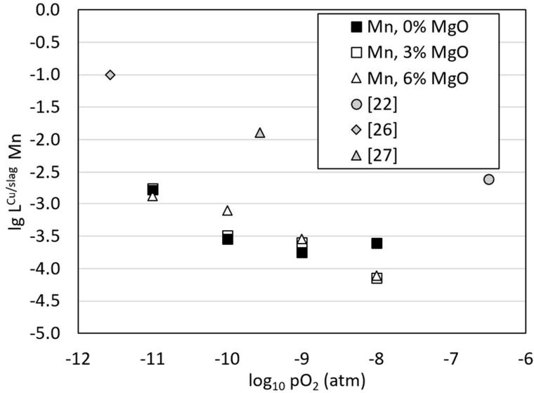
**Figure 7.** The distribution coefficient of manganese between copper alloy and slag as a function of oxygen partial pressure. Results from three earlier studies [22,26,27] have been plotted for comparison.
