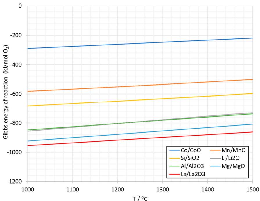
**Figure A1.** An Ellingham diagram for  $\text{Li}_2\text{O}$ ,  $\text{CoO}$ ,  $\text{MnO}$ ,  $\text{La}_2\text{O}_3$ ,  $\text{Al}_2\text{O}_3$ ,  $\text{MgO}$ , and  $\text{SiO}_2$ . Calculated with HSC Chemistry 6.12.
