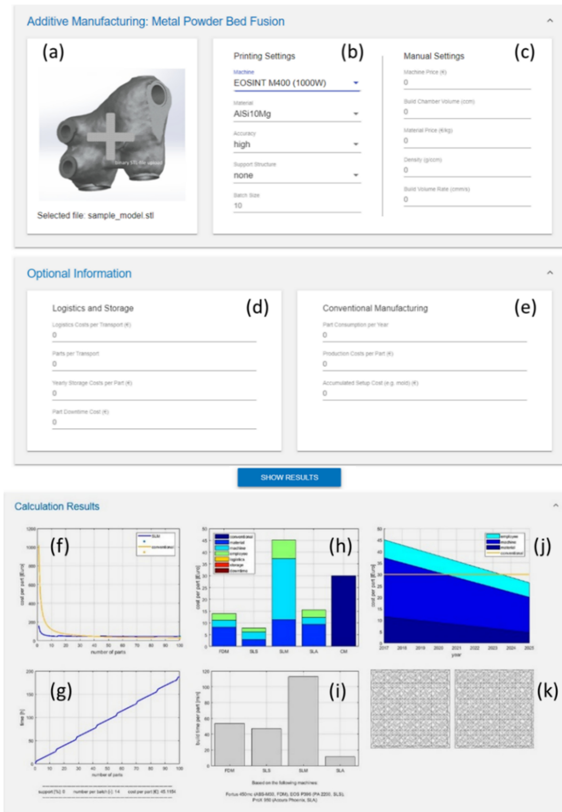
Fig. 6. The graphical user interface of the online tool “amdsp” (additively manufactured digital spare parts) for rapid dimensional, cost and lead time evaluations for metal-based PBF. (a) STL-file upload window, (b) print settings, (c) manual configurations, (d) logistic and storage considerations, (e) possibility to consider comparisons to conventionally produced parts, (f) cost per part analysis, (g) total time function, (h) cost structure comparison for four AM processes and conventional manufacturing, (i) process time comparison for four AM processes, (j) future cost projections, (k) frontal and side part preview.
