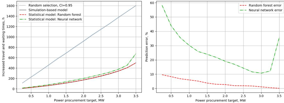
Figure 8: Comparison of methods and statistical model error in increased travel and waiting time compared to the simulation-based model solution.
