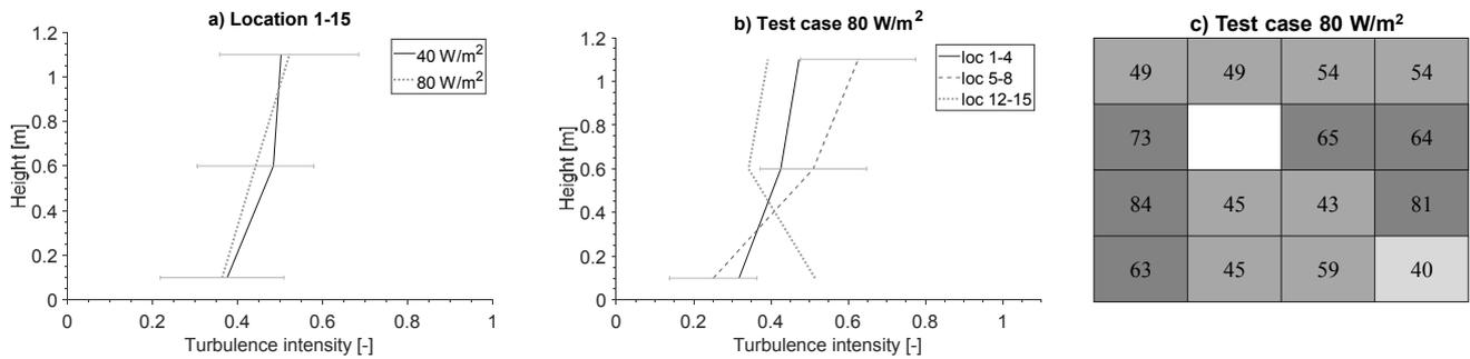
Figure 4. a) The turbulence intensity at C40 and C80, error bars  $\pm$ std. b) The average turbulence intensity in the corridor side (loc. 1-4), middle (loc. 5-8) and window side (loc. 12-15), error bar denotes uncertainty in measurement. c) The maximum turbulence intensity below 1.1 m. The light grey at  $Tu \leq 40$  %, the medium grey at  $40 < Tu < 60$  % and the dark grey at  $Tu \geq 60$  %.
