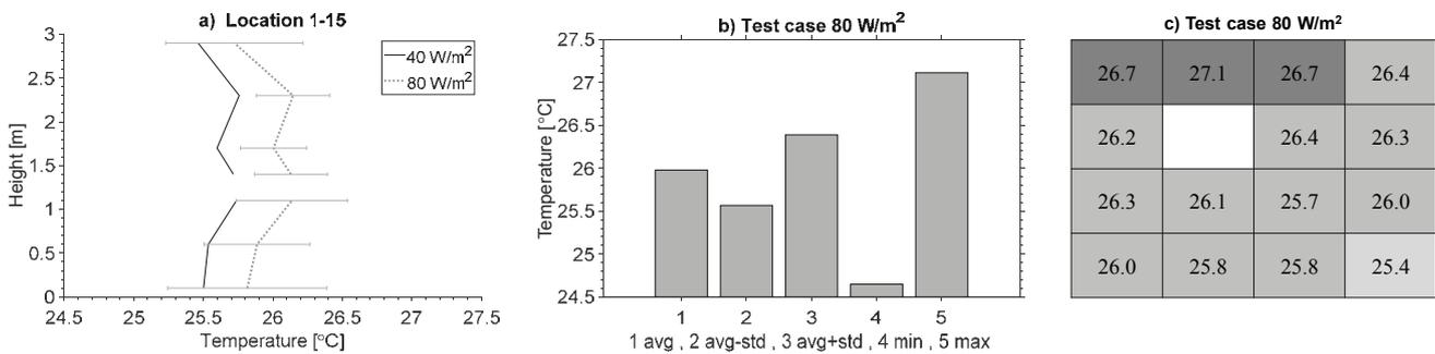
Figure 2. The air temperature: a) The average air temperature at C40 and C80, error bars indicate  $\pm$ std. b) The air temperature statistics at C80. c) The maximum air temperature in the seated person zone below 1.1 m at the locations 1-15 (Figure 1a). The light grey at  $T \leq 25.5^\circ\text{C}$ , the medium grey at  $25.5 < T < 26.5^\circ\text{C}$  and the dark grey at  $T \geq 26.5^\circ\text{C}$ .
