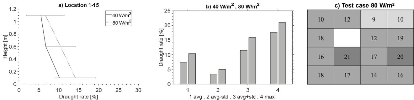
Figure 5. a) The draught rate at C40 and C80 in the seated person zone, error bars  $\pm$ std. b) The statistics of draught rate below 1.1 m. c) The maximum draught rate below 1.1 m. The light grey is category A ( $DR < 10$  %), medium grey is category B ( $DR < 20$  %) and dark grey is category C ( $DR < 30$  %) defined by EN ISO 7730:2005 (CEN, 2005).
