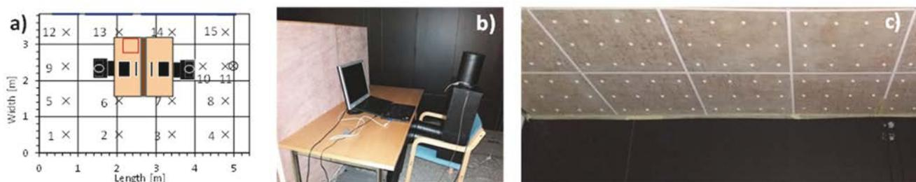
Figure 1. Test chamber: a) the measurement locations 1-15, b) the workstation and c) the diffuse ceiling inlet with the perforation rate of 0.50±0.02 %.
