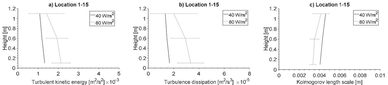
Figure 6. a) The turbulent kinetic energy at C40 and C80. b) The turbulence dissipation at C40 and C80. c) The Kolmogorov length scale at C40 and C80. The error bars denote  $\pm$ std.
