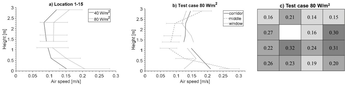
Figure 3. a) The average air speed at C40 and C80, error bar denotes  $\pm$ std. b) The average air speed in the corridor side (loc. 1-4), middle (loc. 5-8) and window side (loc. 12-15), error bar denotes uncertainty in measurement. c) Maximum mean air speed of the locations 1-15 (Figure 1a) below 1.1 m. The light grey at  $\bar{U} < 0.2$  m/s, the medium grey at  $0.2 \leq \bar{U} < 0.3$  m/s and the dark grey at  $\bar{U} \geq 0.3$  m/s.
