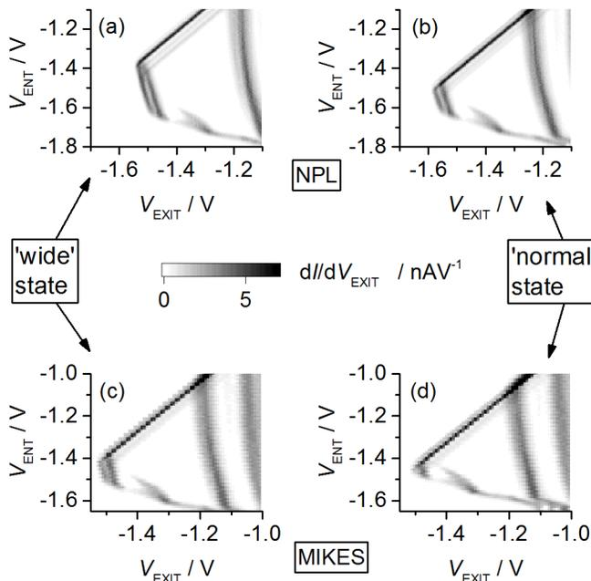
FIG. S6. Pump maps illustrating the ‘wide’ (panels a and c) and ‘normal’ (panels b and d) states exhibited by the pump. Panels (a) and (b) were measured at NPL with  $P_{\text{RF}} = 11.6$  dBm, and panels (c) and (d) were measured at MIKES with  $P_{\text{RF}} = 12.25$  dBm.
