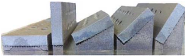
Fig. 5 Rupturing of supports in print job 1
