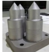
Figure 5a. Printed injection moulding inserts
