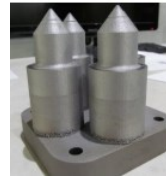
Figure 5a. Printed injection moulding inserts
