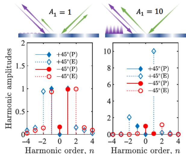
FIG. 8. The amplitudes of excited harmonics for incidences from  $+45^\circ$  and  $-45^\circ$  at  $\omega_0 = \omega_d$ . From left to right, the amplitudes of evanescent mode  $n = +1$  are  $A_1 = 1$ , and  $A_1 = 10$ , respectively. E, evanescent modes; P, propagating modes.
