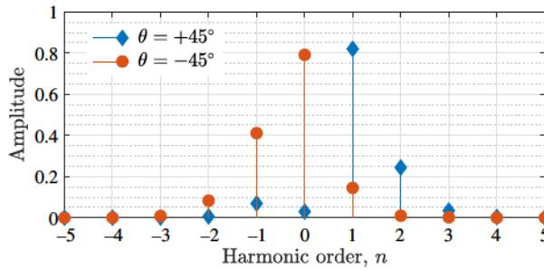
FIG. 12. Distribution of harmonics at  $\omega_0 = 12$  THz for incidence angles  $\theta = +45^\circ$  and  $\theta = -45^\circ$ .  $\beta_M = 5.86 \times 10^5 \text{ m}^{-1}$ ,  $E_{F0} = 1.0 \text{ eV}$ ,  $\tau = 0.5 \text{ ps}$ ,  $a_1 = 0.138$ , and  $a_2 = 0$ . The substrate is assumed to have  $d = 4 \mu\text{m}$  and  $\epsilon_r = 4$ .
