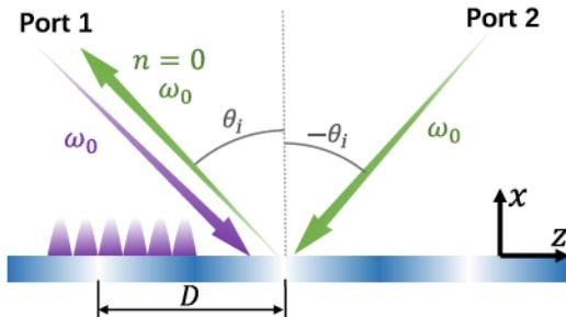
FIG. 2. The metasurface platform for implementing isolators.
