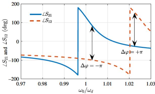
FIG. 6. Transmission phases for waves incident at  $\theta = +45^\circ$  (port 1) and  $\theta = -45^\circ$  (port 2). The surface impedance studied is synthesized with  $b_0 = 39.85 \times 10^{10}$  and  $b_1 = -7.50 \times 10^{10}$ . The spatial period  $D = 0.419\lambda_d$ .
