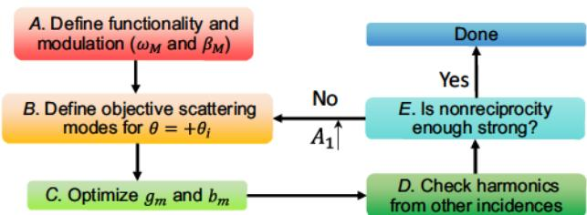
FIG. 4. Block diagram of the design procedure for all exemplary devices proposed in Sec. III.
