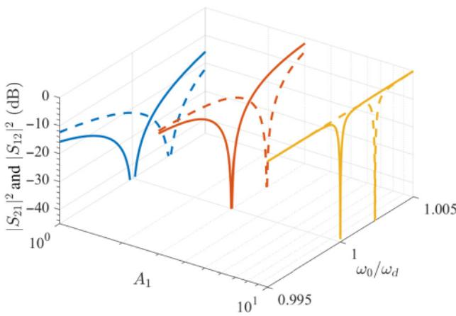
FIG. 3. Transmittances for incidences from port 1 ( $S_{21}$ : solid lines) and port 2 ( $S_{12}$ : dashed lines).  $S_{21} = \Gamma(0, 0)$  for incidence from port 1 and  $S_{12} = \Gamma(0, 0)$  for incidence from port 2. In the three scenarios, the designed amplitudes of the  $n = 1$  evanescent mode are  $A_1 = 1$  (blue),  $A_1 = 3$  (red), and  $A_1 = 10$  (yellow).
