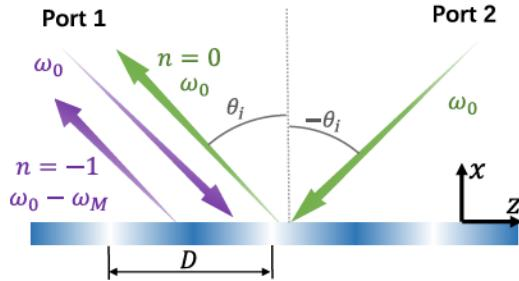
FIG. 7. A quasi-isolator implemented in the proposed metasurface platform.
