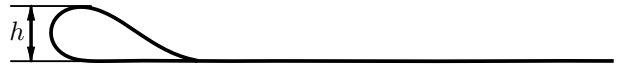
Fig. 2: The folded shape of the strip. The maximum height of the folded strip h depends on the fabric material.
