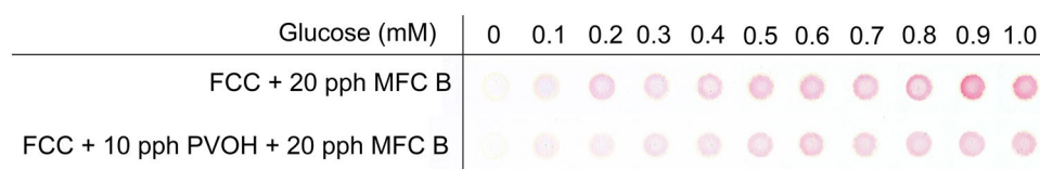
Fig. 8 The colour formation corresponding to glucose concentration in the 4-AAP/DHBS ring experiments
