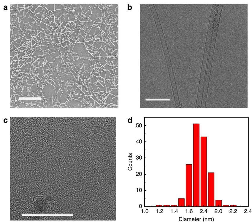
**Figure 3 | SEM and TEM observations of the as-prepared SWCNTs.** SEM (a) and TEM (b,c) image of the as-prepared SWCNTs. Scale bar, 10  $\mu\text{m}$  (a) and 10 nm (b,c). (d) Diameter distribution of the SWCNTs based on TEM observations.
