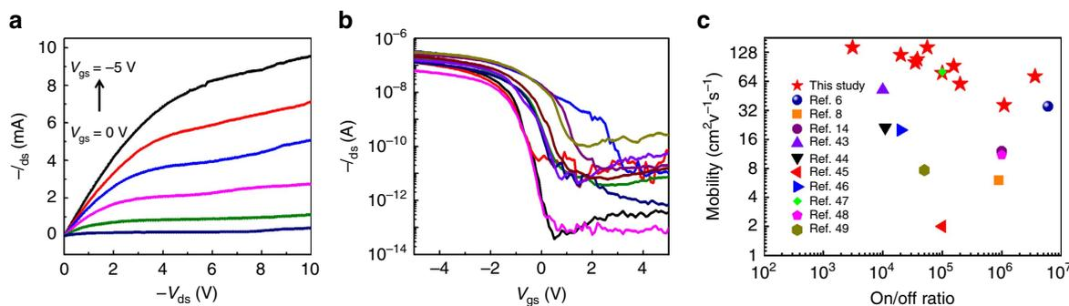
**Figure 6 | Electrical performance of the SWCNT TFTs.** (a) Output ( $I_{ds} - V_{ds}$ ) characteristics of the same device measured at various  $V_{gs}$  from  $-5$  to  $0$  V in  $1$  V step.  $L_{ch} = 200 \mu\text{m}$ ,  $W_{ch} = 100 \mu\text{m}$ . (b) Transfer characteristics of 10 SWCNT TFTs. (c) A comparison of the mobility performance of our SWCNT TFTs with those previously reported.
