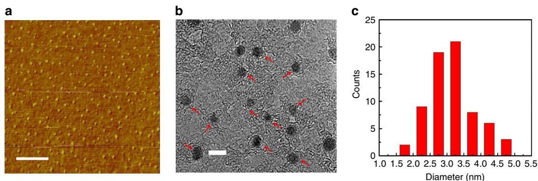
**Figure 2 | Morphology and diameter distribution of the Co nanoparticle partially coated with carbon.** Typical (a) AFM and (b) TEM images of the Co nanoparticles partially coated with carbon, showing that the nanoparticles are monodispersed and uniform in size. The red arrows indicate Co nanoparticles partially coated by a carbon layer. Scale bar, 400 nm (a) and 5 nm (b). (c) A histogram showing the diameter distribution of the nanoparticles based on TEM observations.
