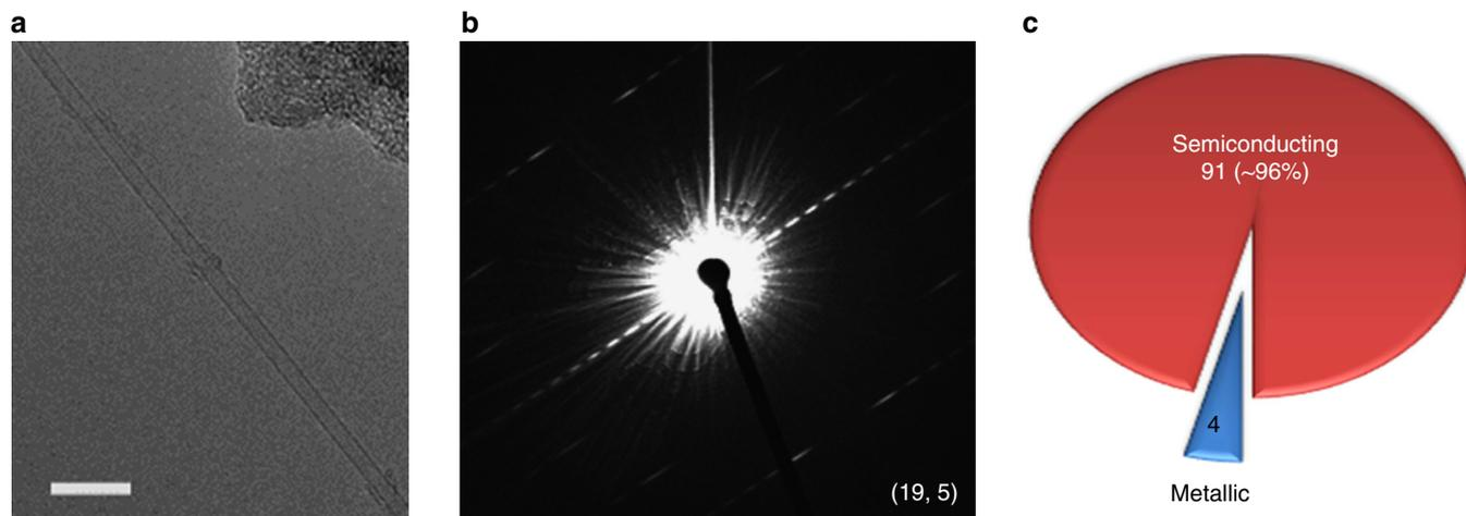
**Figure 5 | Electron diffraction of the SWCNTs.** (a) Typical TEM image of an isolated SWCNT. Scale bar, 10 nm. (b) Electron diffraction pattern of the SWCNT shown in a, the chirality of which is assigned as (19, 5). (c) A pie chart showing the content of s- and m-SWCNTs based on electron diffraction measurements of a total of 95 SWCNTs.
