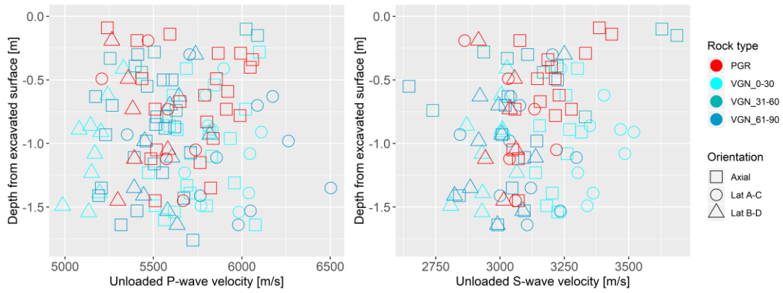
Figure 5. Wave velocities measured unloaded in the axial direction as a function of sampling depth. Left: P-wave velocity; Right: S-wave velocity. Rock type and foliation represented by colour, measurement orientation represented by shape (see Figure 1).
