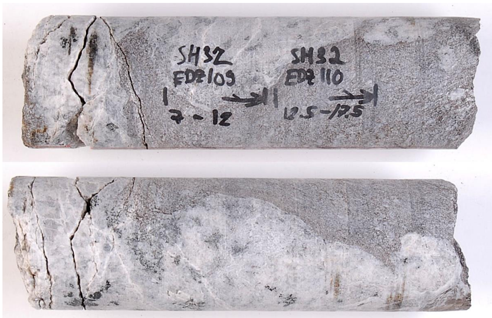
Figure 3: Specimens EDZ109 and EDZ110 showing visible fracturing in the leucosome. The specimens appear as anomalous in plots of S-velocity (as shown in Figure 2), P/S –ratio, Poisson’s ratio, shear impedance and Poisson impedance in respect to depth from the excavated surface. Adapted from Kiuru (2017).
