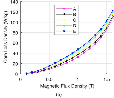
Fig. 4: Measured core loss curves of different width samples at (a) 50 Hz (b) 400 Hz.
