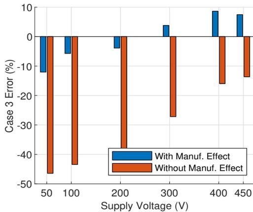
Fig. 12: Error in the stator core losses with and without considering the manufacturing effects in Case 3 (laser cutting, welding and shrink fitting) at 50 Hz and different supply voltages. Laser cut welded stator is measured with frame.
