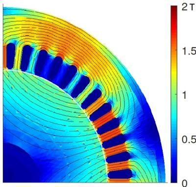
Fig. 10: Flux density distribution at 400V and 50 Hz supply. The color discontinuities are only artifacts due to the plotting routines.
