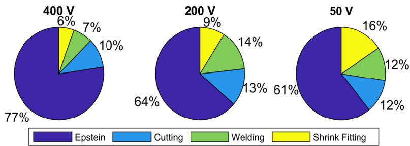
Fig. 11: Impact of manufacturing processes on stator core losses at 50 Hz supply frequency. Core losses from standard Epstein frame test is calculated as P1. Laser cutting, welding and shrink fitting effects are calculated by differences P2-P1, P3-P2 and P4-P3 respectively.
