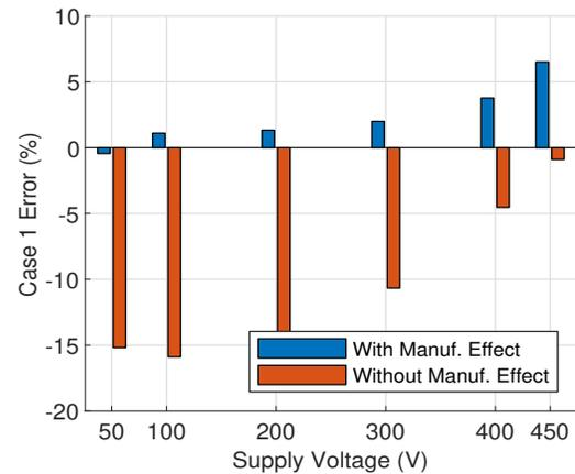
Fig. 13: Error in the stator core losses with and without considering the manufacturing effects in Case 1 (only welding effects) at 50 Hz and different supply voltages. EDM cut welded stator is measured without frame.
