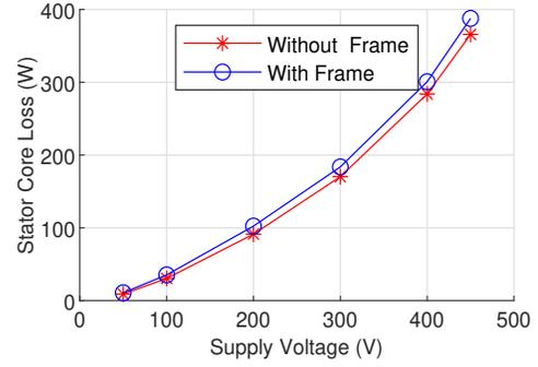
Fig. 8: Measured stator core losses with and without shrink fit at 50 Hz and different supply voltages.
