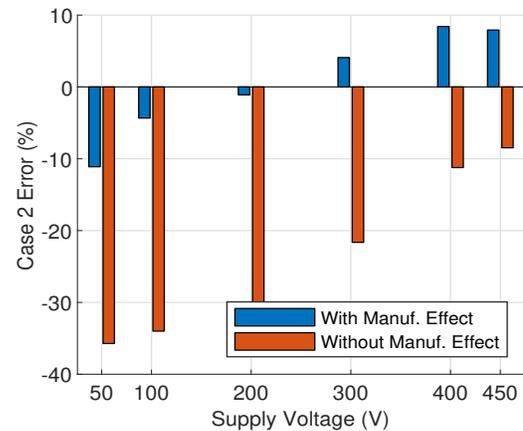
Fig. 14: Error in the stator core losses with and without considering the manufacturing effects in Case 2 (only laser cutting and welding) at 50 Hz and different supply voltages. Laser cut welded stator is measured without frame.
