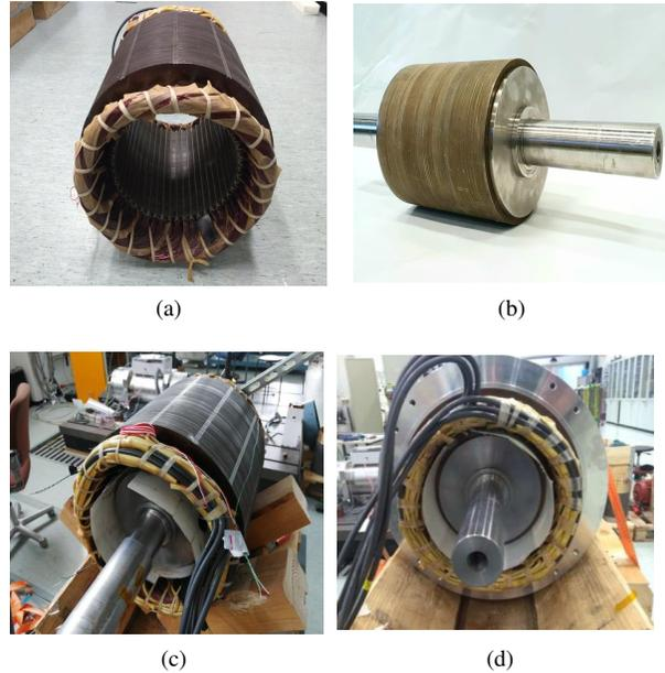
Fig. 2: Dummy blocked rotor setup. (a) wounded stator (b) laminated rotor without rotor slots and conductors (c) stator without frame (d) stator with frame.
