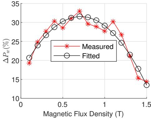
Fig. 7: % Difference in the core loss density due to the welding effect at 50 Hz. Fitting is done with a polynomial of second order.
