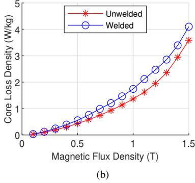
Fig. 6: Magnetic measurements of unwelded and welded ring core samples at 50 Hz (a) magnetization curve (b) core loss measurements.
