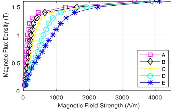
Fig. 3: Measured magnetization curves at 50 Hz for different sample widths. The detail of samples are provided in Table I.
