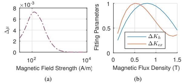
Fig. 5: Parameters (a)  $\Delta\mu$  (b)  $\Delta K_h$  and  $\Delta K_{ex}$  in per units. The maximum values of  $\Delta K_h$  and  $\Delta K_{ex}$  are 0.023 and 0.0022 respectively. In general effect of cutting diminishes at saturation.
