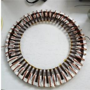
Fig. 1: Ring core assembled from the stator laminations.
