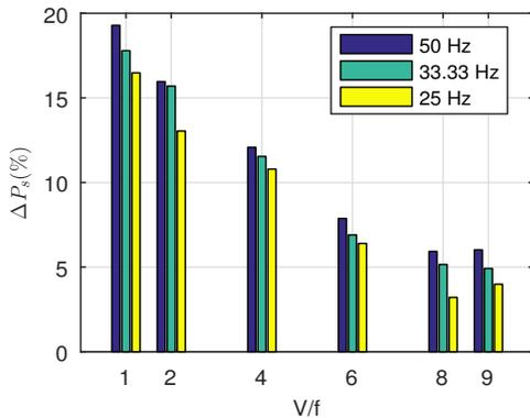
Fig. 15: Effect of shrink fitting on the measured stator core losses at different supply voltages and frequencies. V/f ratio is kept same across different frequencies.
