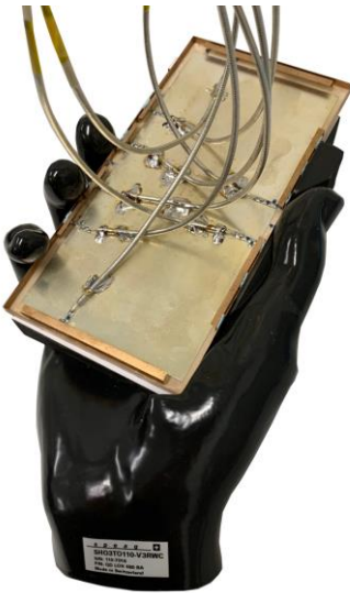
Fig. 5 Antenna prototype and the hand phantom.
