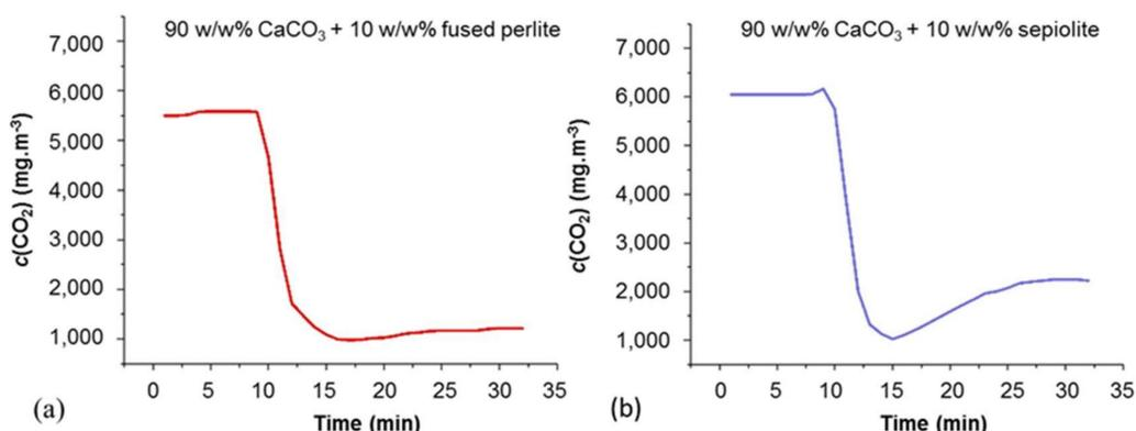
Figure 29. CO<sub>2</sub> in situ capture in (a) fused perlite, and (b) sepiolite blended at 10 w/w% with CaCO<sub>3</sub> (GCC).
