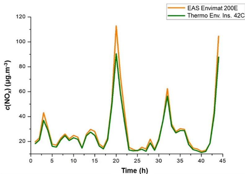
**Figure 19.** Comparison of ambient  $\text{NO}_x$  concentrations (Faculty of Technology and Metallurgy (FTM), University of Belgrade, sampling point) between chemiluminescence  $\text{NO-NO}_2\text{-NO}_x$  analysers: Thermo Environmental Instruments 42C (green line) vs. EAS Envimet ČR, č.r.o. 200E (orange line).
