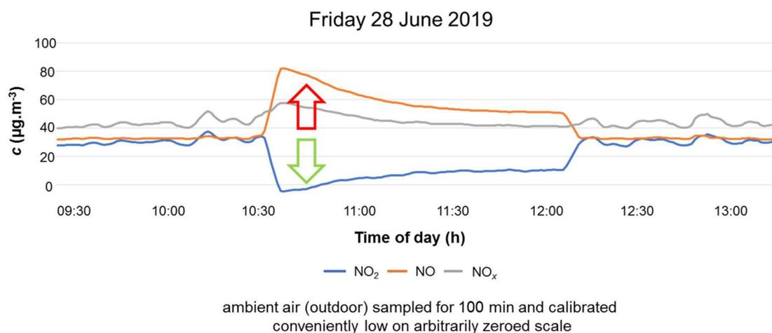
**Figure 22.** Insertion of the box design surface flow filter in the stream of externally sampled air. The red arrow indicates the generation of NO while the green arrow indicates  $\text{NO}_2$  concentration and drops during the period of exposure.
