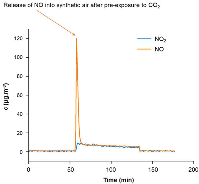
Figure 31. The release of selectively intercalated NO from sepiolite upon exposure to CO<sub>2</sub>.
