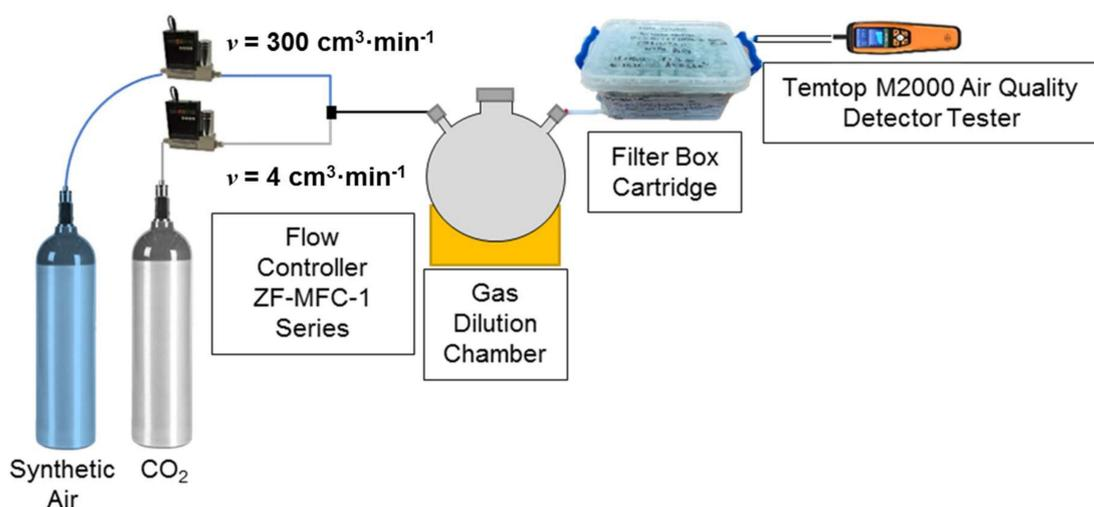
Figure 30. Illustration of the method for sequential exposure to CO<sub>2</sub> and flushing with synthetic air.
