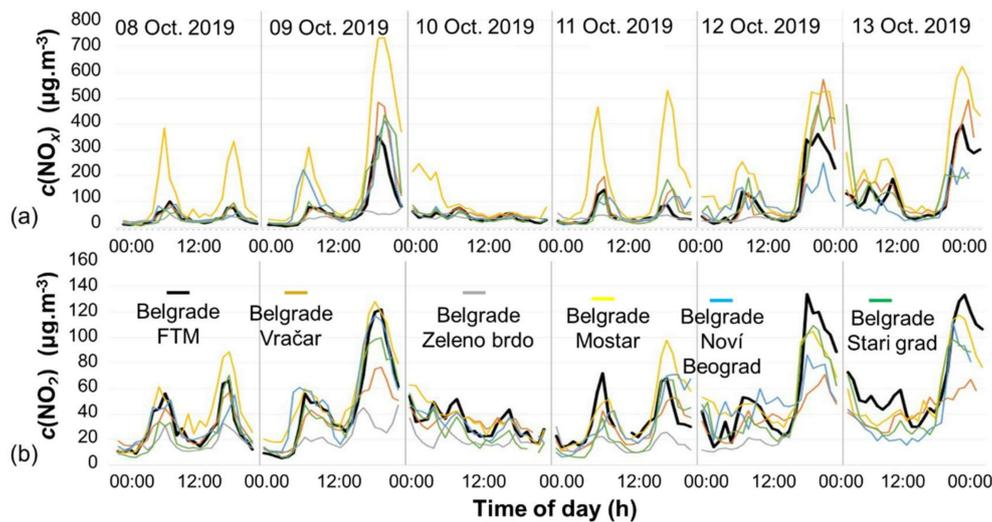
**Figure 18.** Monitoring of (a) total  $\text{NO}_x$  and (b)  $\text{NO}_2$  levels to compare official data from a range of monitoring stations with laboratory sampling of external air at the Faculty of Technology and Metallurgy (FTM), Belgrade (1-h mean values).
