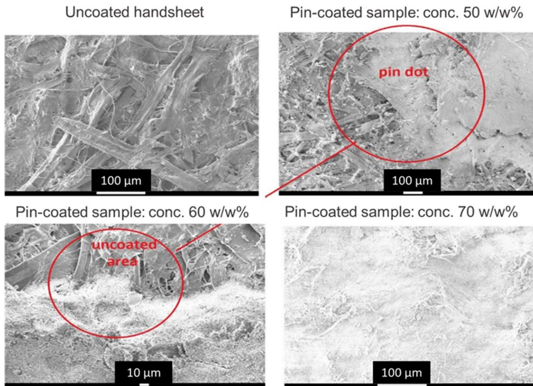
**Figure 11.** The scanning electron microscope (SEM) images of the surface of pin coated substrate showing applications made at medium and high solids content (50 w/w%, 60 w/w%, and 70 w/w%, respectively)—different magnifications are used conveniently to demonstrate both the coating dot edge line and individual coating structure.
