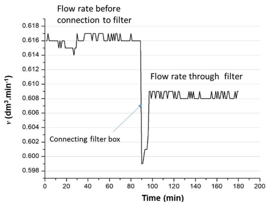
**Figure 21.** Ambient outdoor airflow rate before and during connection to the filter.
