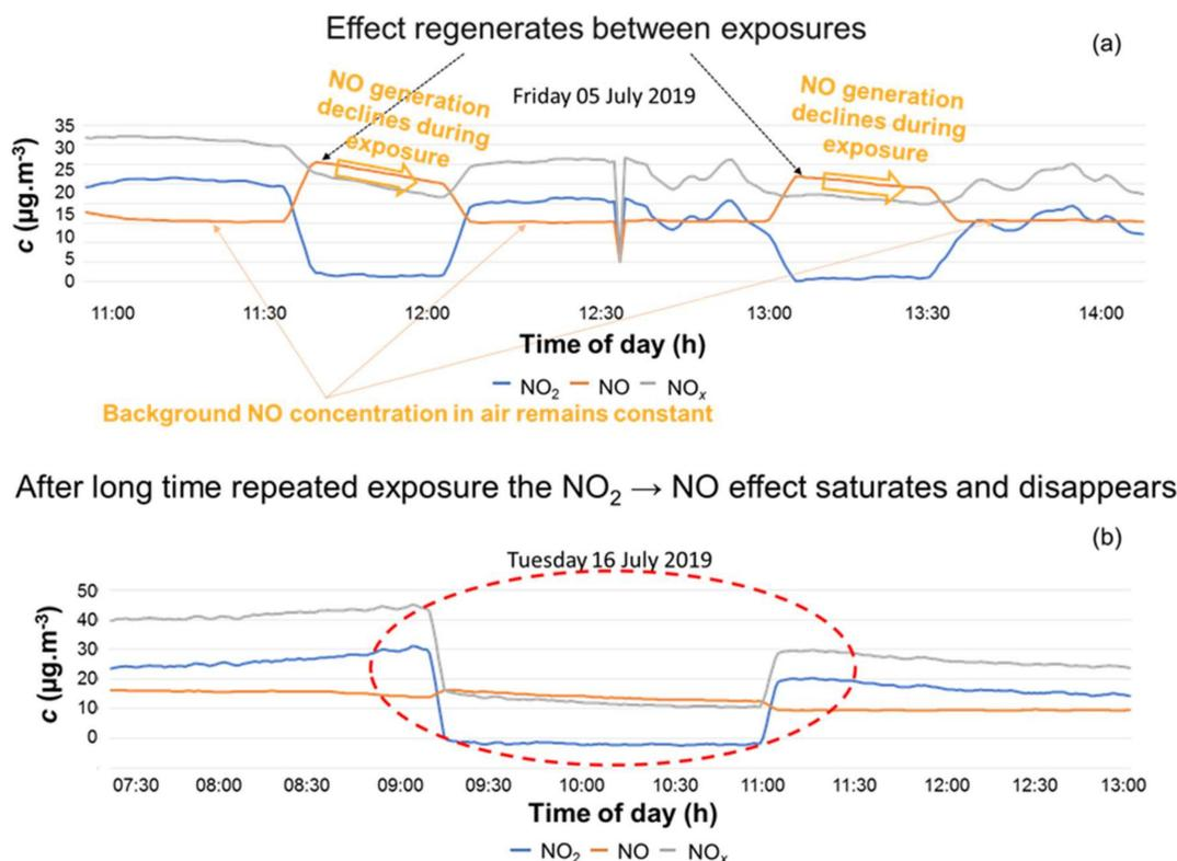
**Figure 23.** (a) Regeneration of the NO<sub>2</sub> → NO effect between exposures while background NO level in the incoming air is constant, (b) long time repeated exposure (as shown Friday 5th July–Tuesday 16th July 2019) saturates the RedOx reaction.
