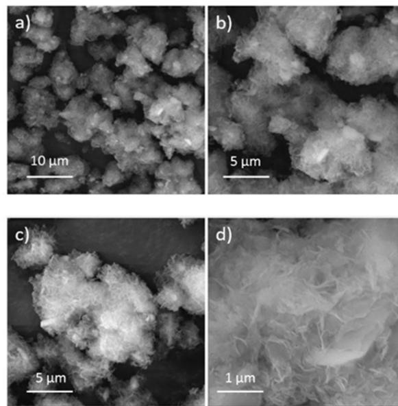
**Figure 14.** FESEM images showing the typical high surface area structure of hydroxyapatite (HAP) at increasing magnification (see scale bars) (a–d).
