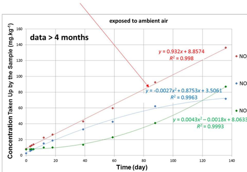
**Figure 12.** Initial results of the exposure of CaCO<sub>3</sub> to ambient air over several months, which revealed a conversion reaction of  $-\text{CO}_3^{2-}$  to  $-(\text{NO}_2^-/\text{NO}_3^-)_2$  rather than simple inert surface adsorption data.
