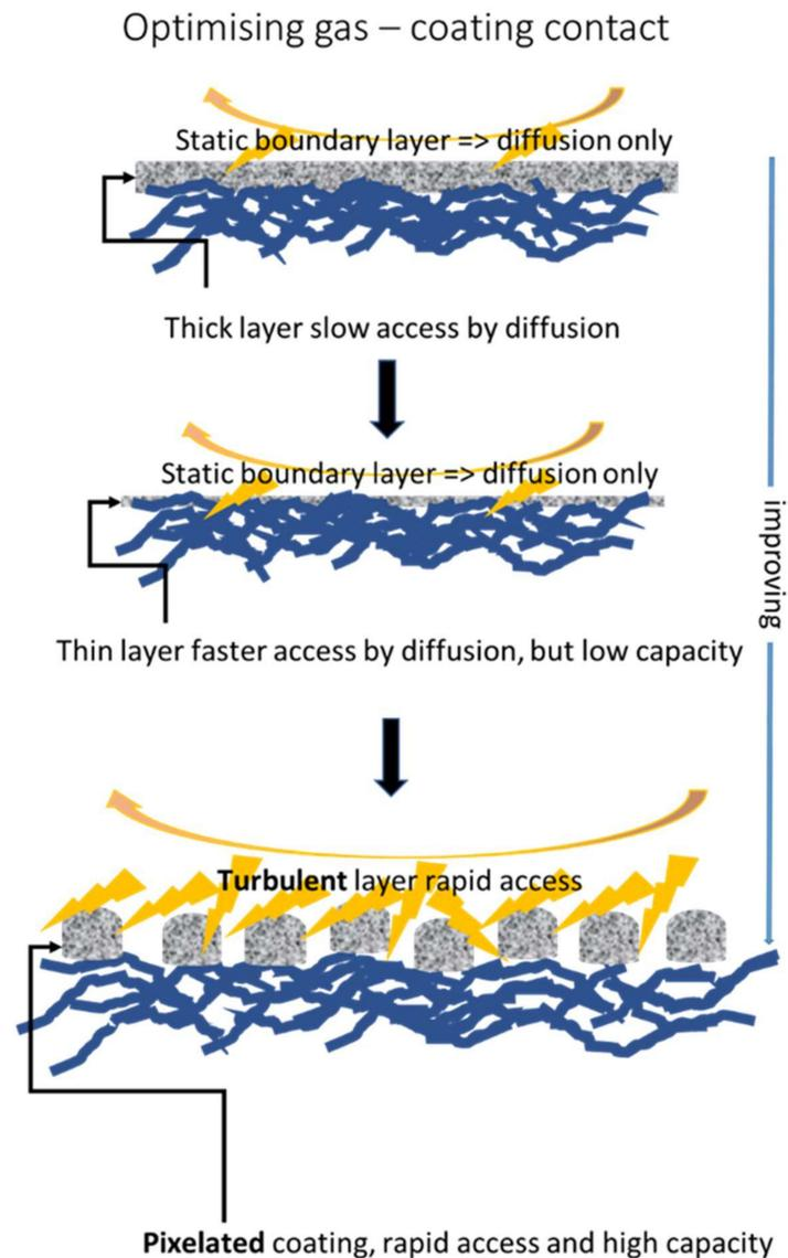
**Figure 9.** Illustration of the need for and methods that can be used to optimise gas-coating contact.
