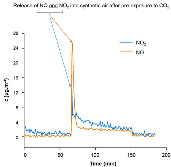
Figure 32. Non-selective pore sorption of NO<sub>x</sub> components resulted in their release on exchange with CO<sub>2</sub>.
