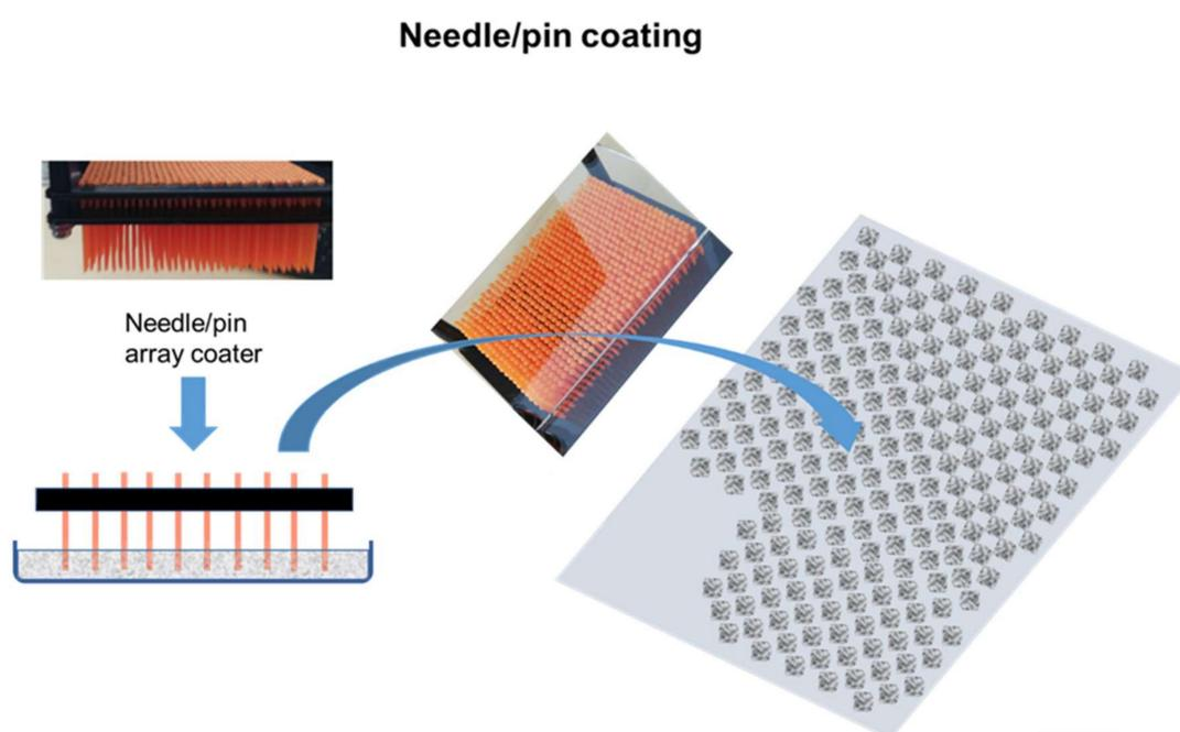
**Figure 10.** A hand-held pin coater and an illustration of its application to produce a pixelated coating on the fibrous substrate.
