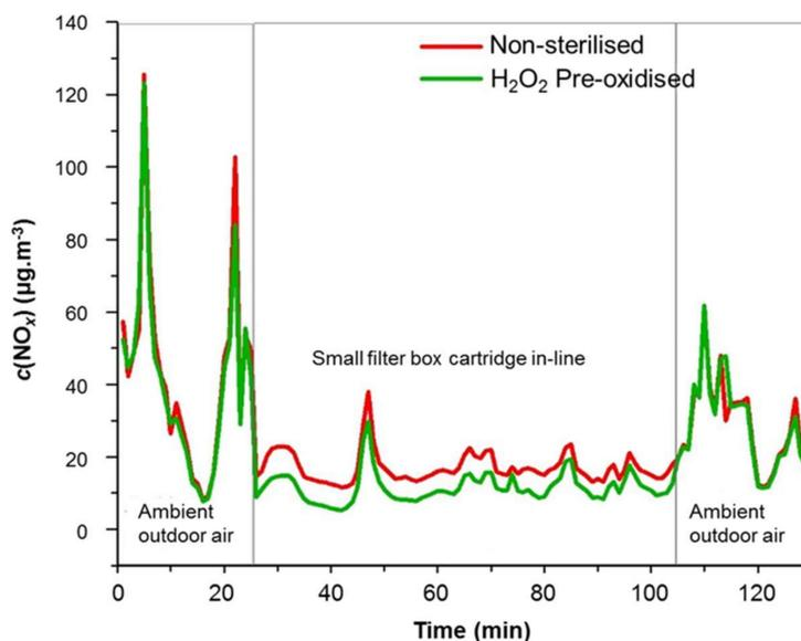
**Figure 27.** Filter efficiency comparison between H<sub>2</sub>O<sub>2</sub> pre-oxidised (green line) and non-sterilised (NO<sub>2</sub> → NO conversion, red line) samples mounted in the smaller filter box.
