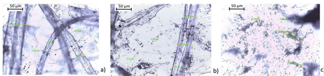
**Figure 8.** Optical microscope images present the mix of micro nano-fibrillated cellulose (MNFC) and  $\text{CaCO}_3$  particles that were used in coatings: (a) and (b) fibres of recycled newsprint sheet (NP), and (c) dispersion of  $\text{CaCO}_3$  in the matrix of  $\text{MNFC}_{\text{NP}}$ .
